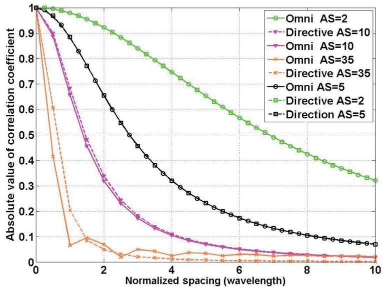
FIGURE 2: This graph illustrates throughput performance of a MIMO system based on the channel correlation of various properties. Both the theoretical measurements of these properties and their effect on system performance are shown. While radiation pattern does not play a large role in correlation, antenna spacing and the angular spread of the antennas do have a large effect on correlation.
