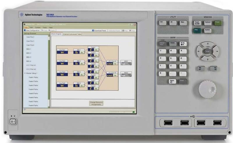
FIGURE 1: The N5106A PXB Baseband generator and channel emulator provides up to 4 baseband generators (BBGs), 8 faders, the industry's widest bandwidth of 120 MHz, custom MIMO correlation settings (e.g., predefined channel models, antenna pattern and correlation matrix), and supports testing and troubleshooting of 2x2, 2x4, and 4x2 MIMO.
