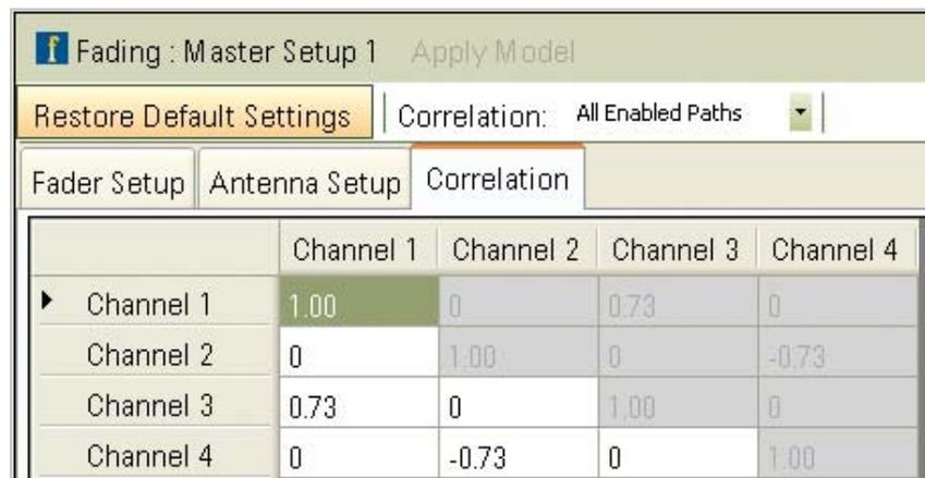
FIGURE 4: Using the PXB's correlation screen, the engineer can set path-to-path correlation or channel-to-channel correlation for all paths within each fader.
