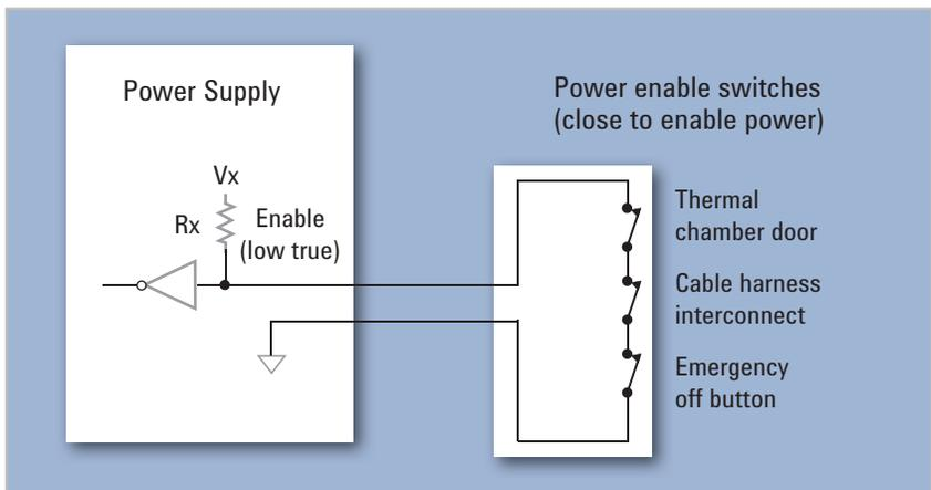
Figure 2. Remote enable should be self-biased and require a short circuit to enable the supply.
