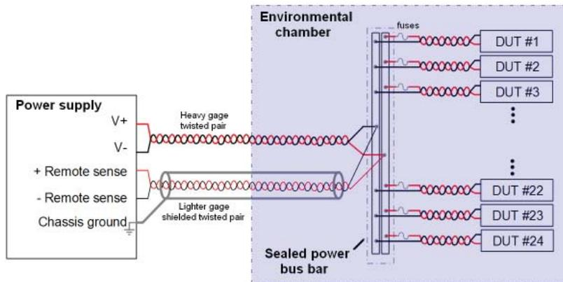
Figure 1. Power system for life and durability testing
