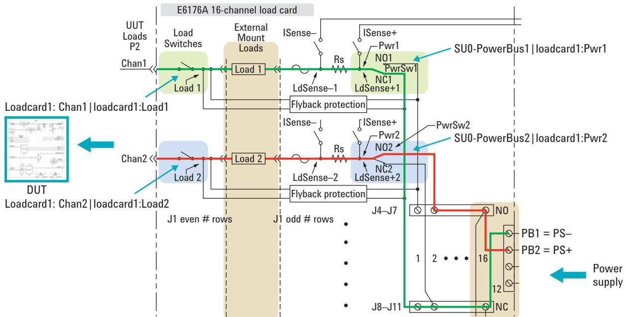
Figure 9. Block diagram showing the switching path connections via load card
