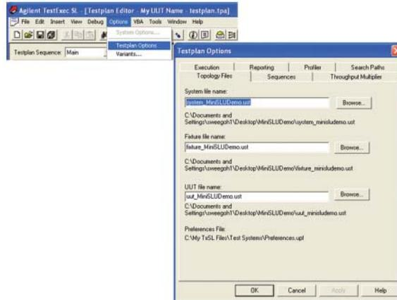
Figure 6. Specifying the switching topology layers for a testplan
