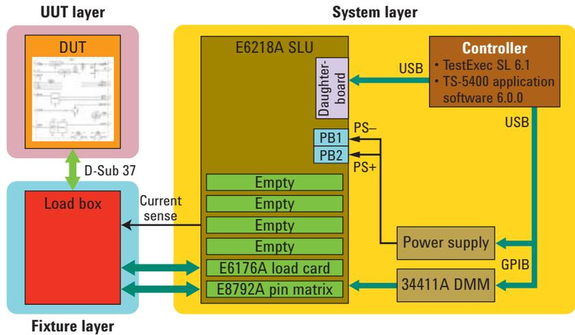
Figure 1. System block diagram showing system, fixture and UUT layers
