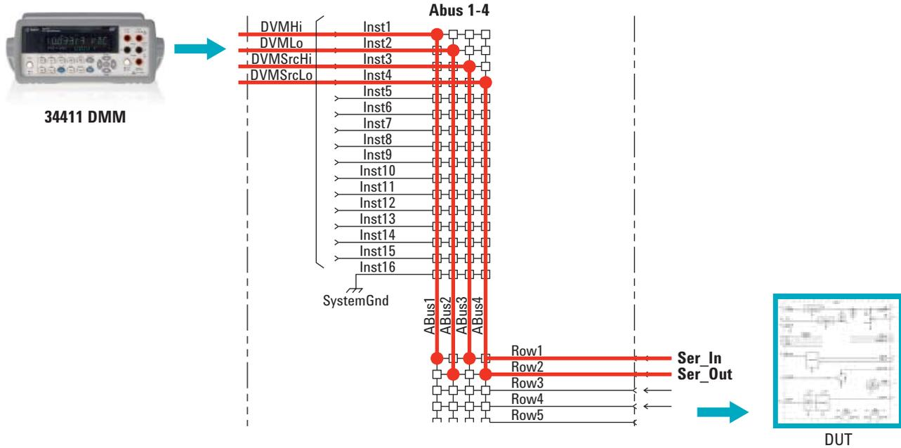
Figure 8. Block diagram showing the switching path connections via pin matrix card
