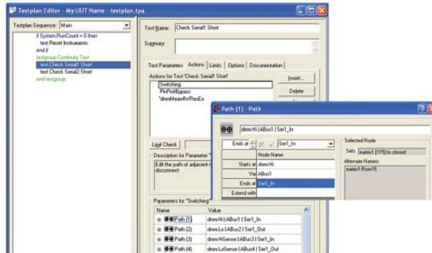
Figure 7. Specifying the switching paths in a test
