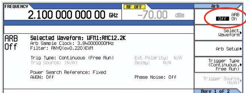
Figure 5. Select waveform "RMC12.2K" and turn arb off
