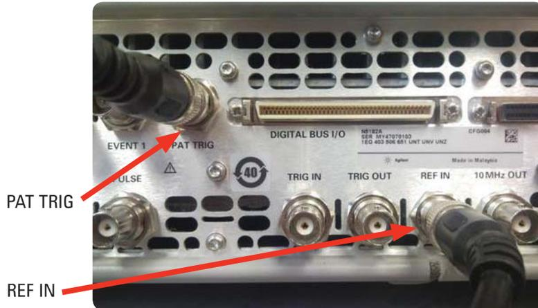
Figure 2. MXG signal generator rear panel connections
