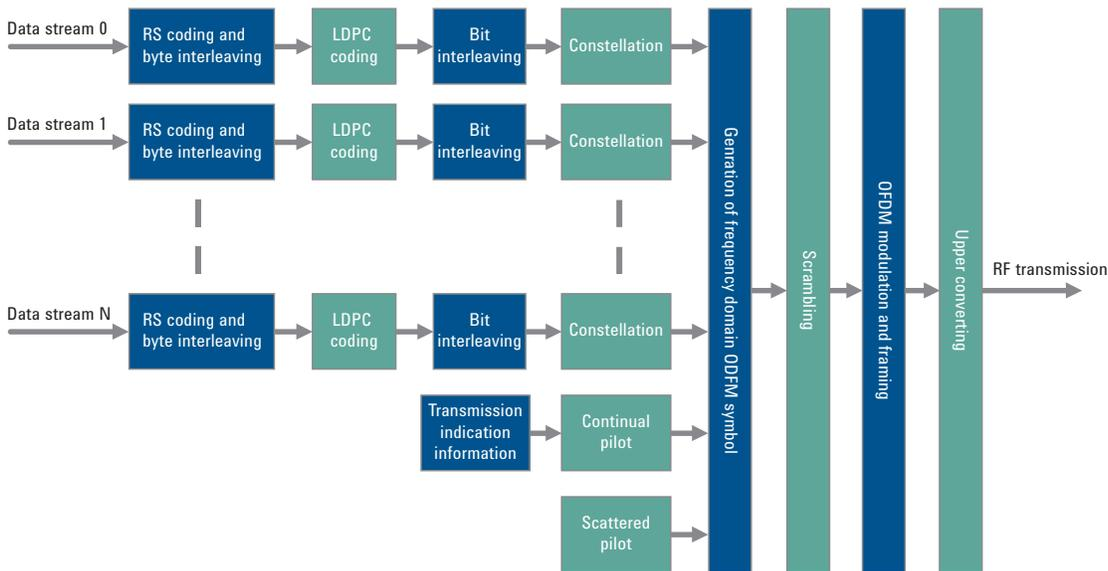
Figure 1. CMMB block diagram.
