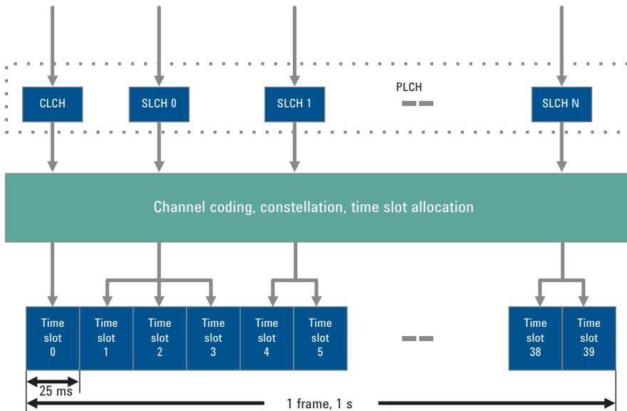
Figure 2. Logical channel structure.
