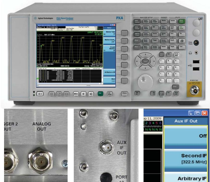
FIGURE 1: The PXA features super-wide IF technology and outstanding measurement accuracy,  $\pm 0.19$ -dB accuracy and a low noise floor DANL of  $-172$  dBm with preamp ( $-160$  dBm with no preamp) at 2 GHz for superior useable dynamic range. Compatibility is enhanced with a flexible analog output and a selectable-frequency IF output.
