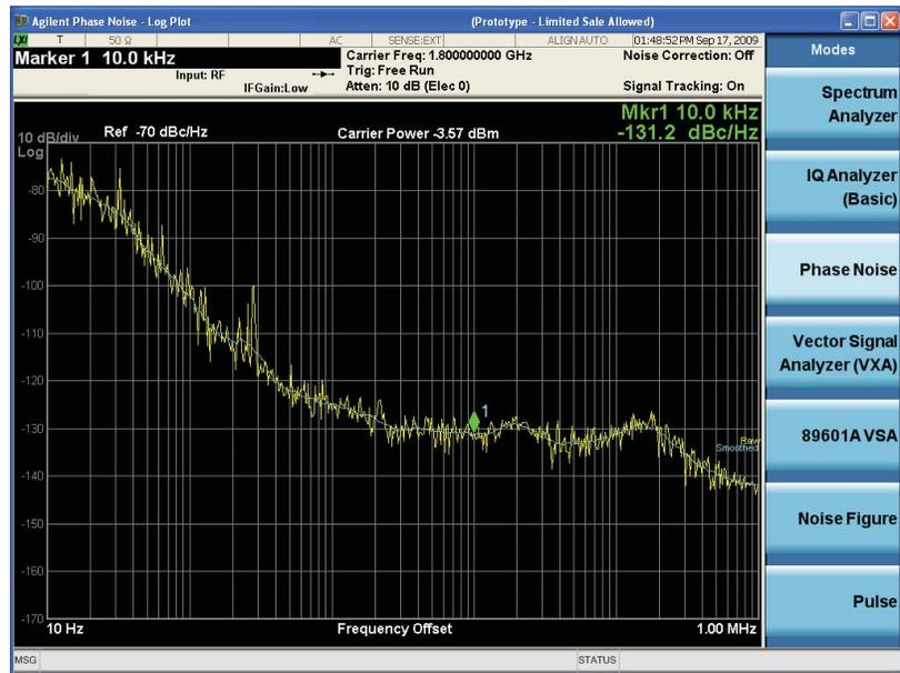
FIGURE 2: This measurement reflects the built-in functionality and the performance of the Agilent PXA (using an external reference), where a fast and automatic phase noise measurement yields  $-131$  dBc/Hz at  $10$  kHz and  $-77$  dBc at  $10$  Hz, at a carrier frequency of  $1.8$  GHz.
