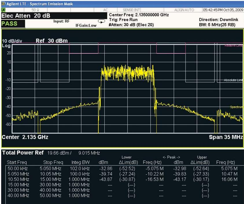
Figure 22. Spectrum emission mask measurement for 10 MHz E-TM 1.1 signal
