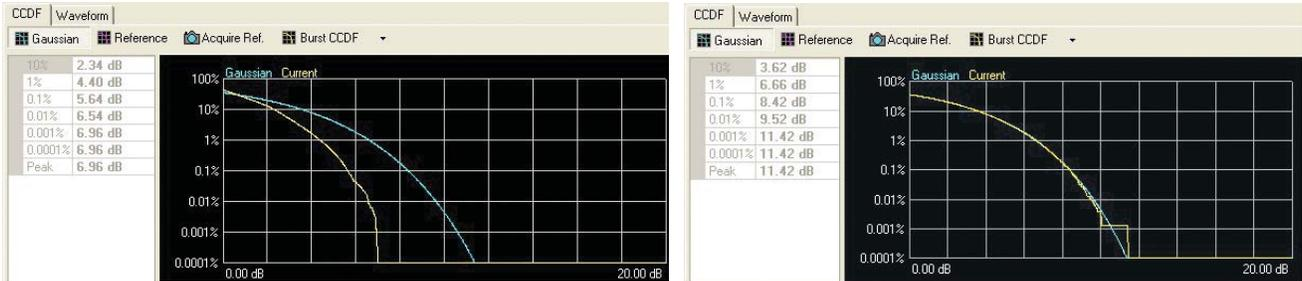
Figure 14. CCDF for 5 MHz fully allocated uplink signal (left) and downlink signal (right)
