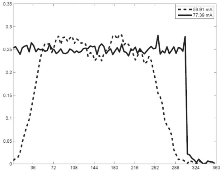
Figure 12. Precise top-up produces a square, even fill pattern that ensures a constant intensity radiation source for experiments
