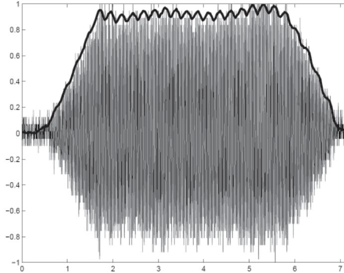
Figure 8. Comparison of fill-pattern measurements made with the capacitive-strip recorder (thin oscillating lines) and the FHP (thick line)
