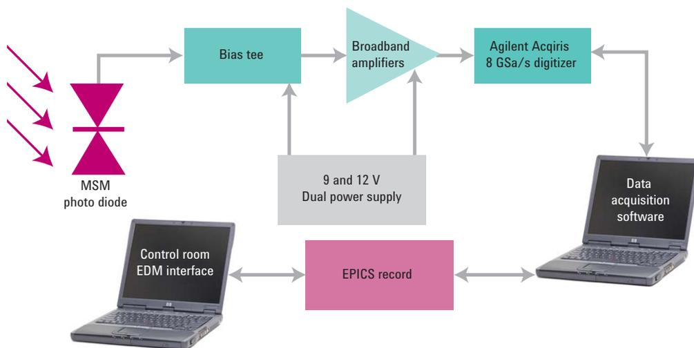
Figure 7. Experimental setup for measurement of fill pattern
