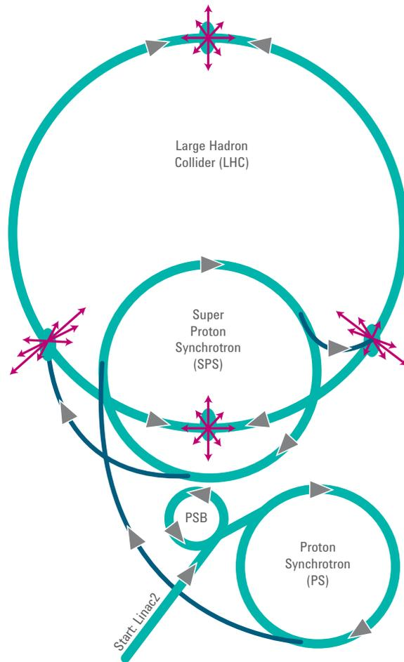
Figure 1. Simplified diagram of the LHC multi-stage synchrotrons as used to accelerate protons
