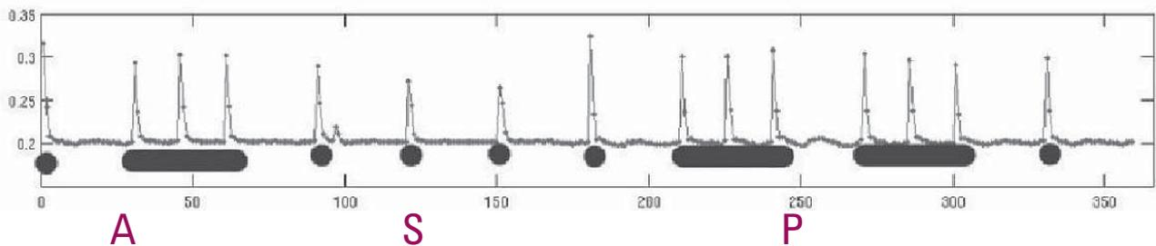
Figure 11. Morse code dots and dashes were formed by injecting electrons into arbitrary RF buckets
