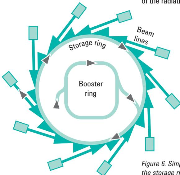
Figure 6. Simplified diagram of the Australian Synchrotron: the booster ring (inner) feeds the storage ring (outer) and beamlines (branches from storage ring) house experiments
