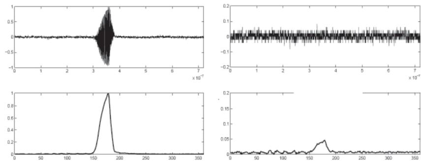
Figure 9. Comparison of fill-pattern measurements made during controlled loss of beam. The lower-right trace shows that the FHP was able to measure a lower-level remnant fill pattern.
