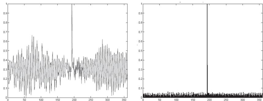
Figure 10. Comparison of first shot into storage ring (left) and finished injection test (right), showing all injected current in the correct RF bucket
