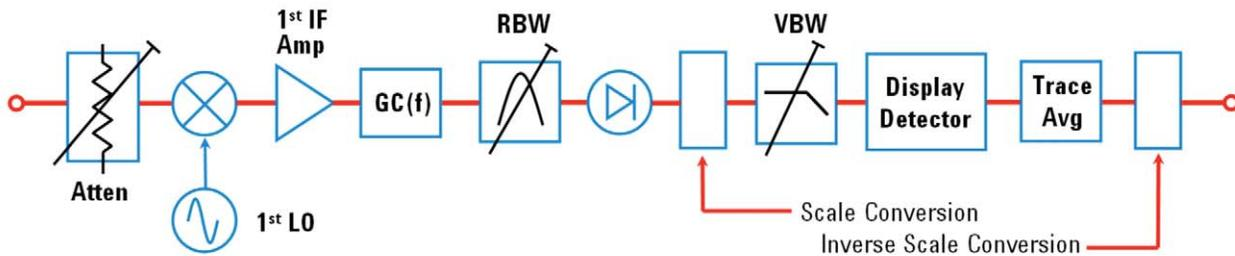
Figure 8. Low band measurements are made by upconverting the signal, then correcting for frequency response flatness with the block labeled  $GC(f)$ . This block diagram is particularly easy to model for noise.
