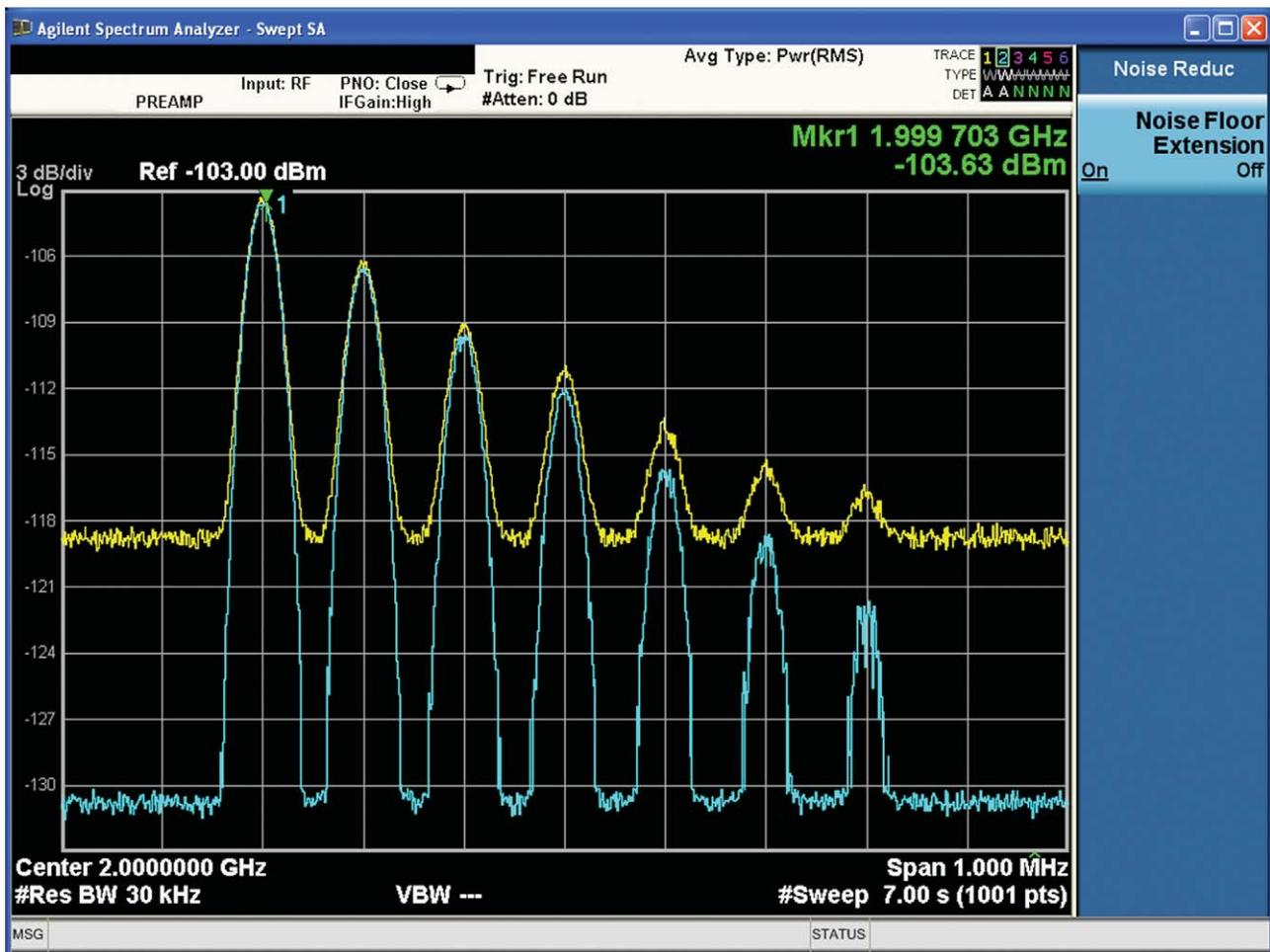
Agilent's Noise Floor Extension technology can provide up to 12 dB improvement in analyzer noise floor, revealing some previously hidden signals and allowing other to be more accurately measured.
