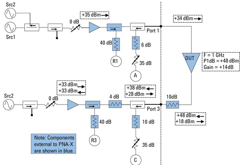
FIGURE 2: Block diagram modifications for testing +48 dBm amplifier.
