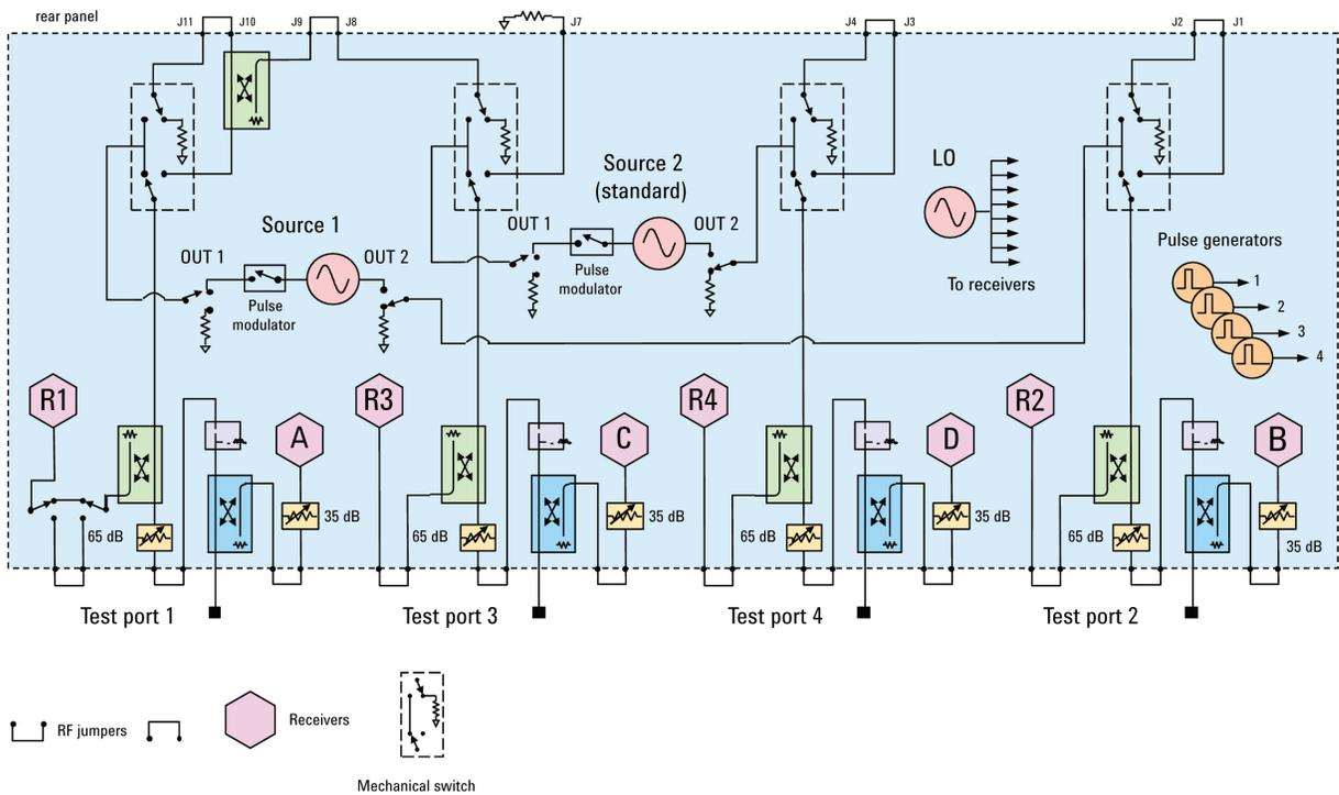
FIGURE 1: Block diagram of the PNA-X N5242A Option 423 RF test set.
