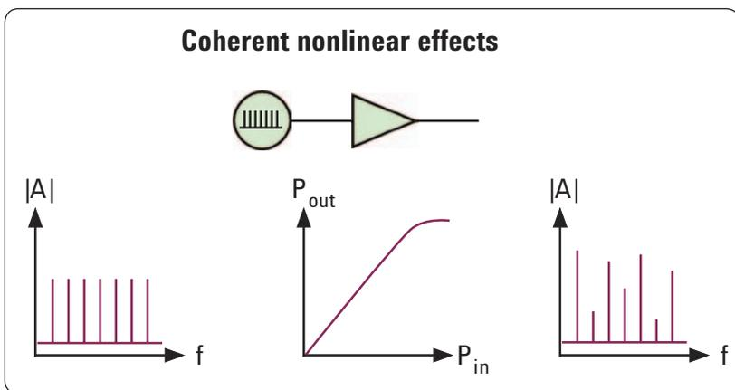
Figure 3. Nonlinear products can combine in unpredictable ways in coherent systems.
