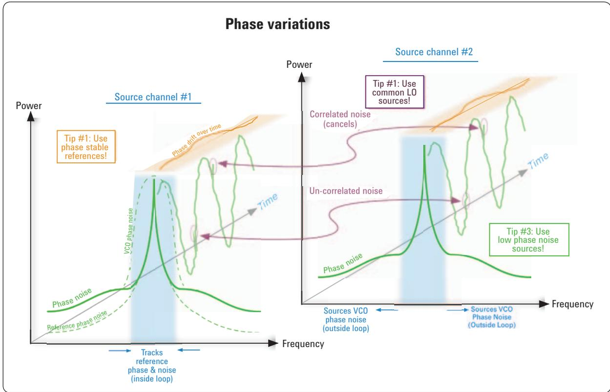
Figure 5. Phase variations between reference-locked signal sources track within the limits of loop bandwidth of their PLLs. Performance is improved by using high quality stable references and instruments with low phase noise, or by locking higher-frequency references or LOs.
