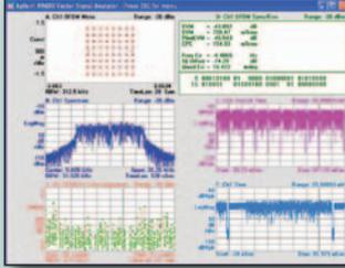
The Agilent 89601A vector signal analysis software is a flexible tool that includes analysis options for a wide range of common modulations. The VSA software is supported on a number of platforms including multi-channel oscilloscopes, multi-channel vector signal analyzers, and most Agilent spectrum analyzers. The software can make a variety of multi-channel measurements including built-in measurements for cross correlation, coherence and cross spectrum.
