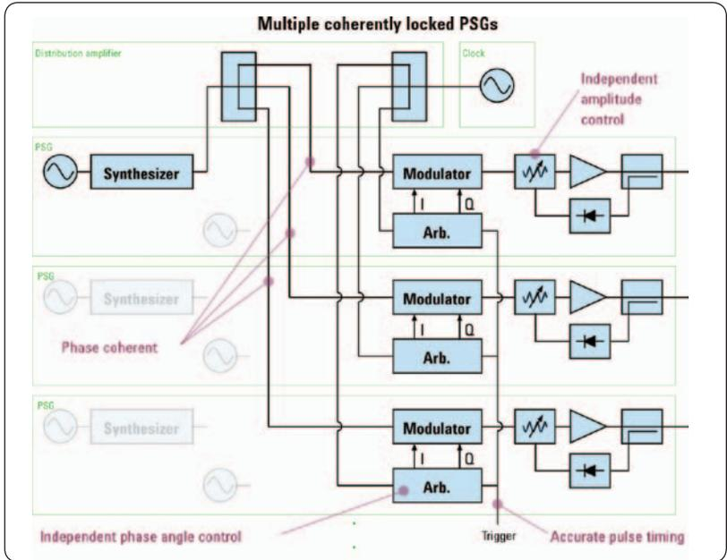
Figure 17. Simplified block diagram of coherently locked and synchronized PSG vector signal generators.
