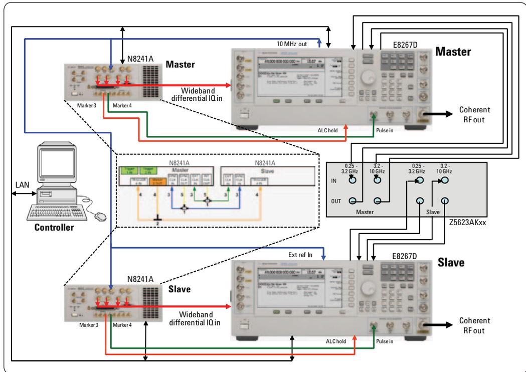
Figure 18. These are the connections for two coherent wideband VSGs using an E8267D PSG and an N8241A external AWG.
