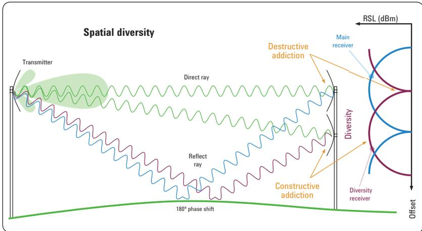
Figure 1a. The coherent nature of multi-path signals causes them to combine constructively or destructively. A spatial-diversity antenna ensures good reception in a multi-path environment by using spatially separated antennas.
