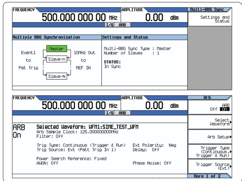
Figure 14. MXG with Option 012 includes the Multi-BBG Synchronization feature, which is used to align the BBGs. One instrument should be designated as master and the others as slaves.
