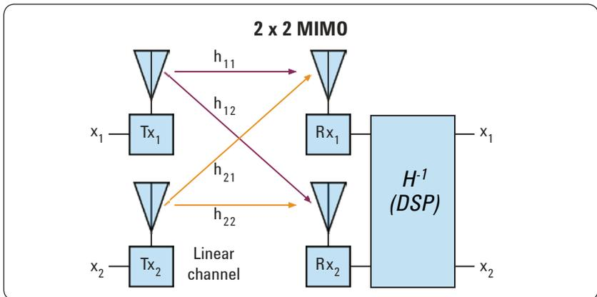
Figure 1b. MIMO systems use multiple antennas, space-time coding and channel-estimation algorithms to create multiple spatial data channels capable of uniquely transmitting data.
