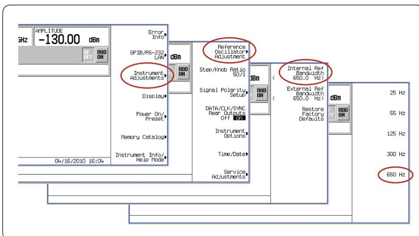
Figure 10. The reference bandwidth setting on the PSG with Option UNX should be set to the widest setting for best phase stability between reference-locked instruments.
