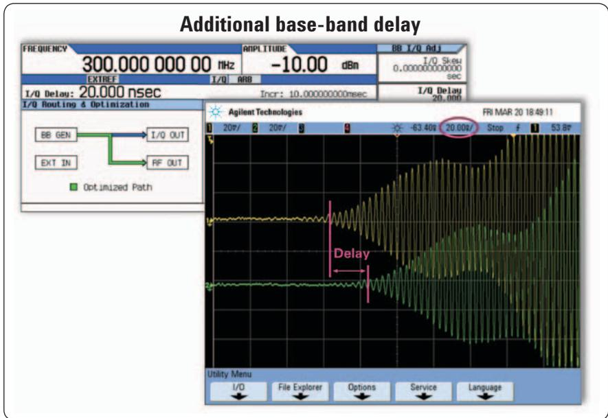
Figure 15. MXG with Option 012 includes Multi-BBG Synchronization feature used to align the BBGs. Each instrument should be designated as master or slave.
