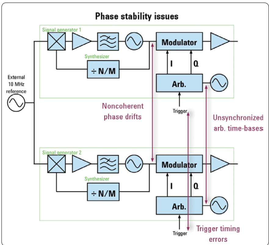
Figure 4. Locking the 10 MHz references of multiple sources provides only limited phase stability between instruments.
