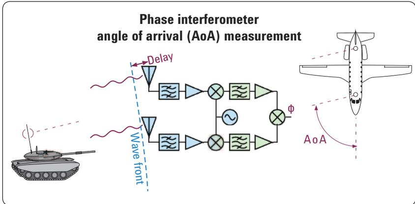
Figure 1e. A direction-finding system can determine the angle of arrival of a transmitted signal by measuring the phase delay at two spatially separated receivers.
