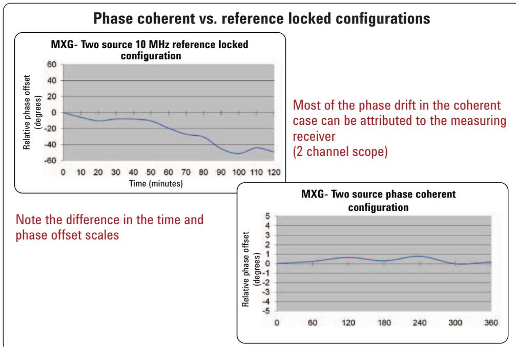
Figure 7. Measured phase drift of two 10 MHz-locked MXG signal generators compared to two coherently-locked MXGs (sharing a common LO).
