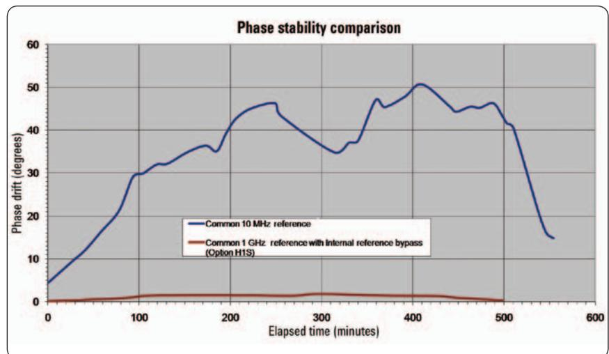
Figure 12. Phase drift comparison of PSGs with 10 MHz reference locked versus 1 GHz references locked (Option H1S).
