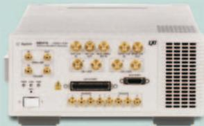
The Agilent N8241A arbitrary waveform generator combines the unprecedented performance of Agilent's AWGs with the unsurpassed flexibility of scalable modules. High sampling rates of either 1.25 GSa/s or 625 MSa/s, and high bit resolution enable designers to create ideal waveforms for accurate test of radar, satellite, digital-radio and frequency-agile systems.
