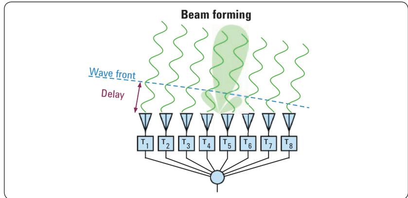
Figure 1c. A phased array of antennas forms a beam by adjusting the phase between coherent antennas such that the signals constructively combine in the desired direction and destructively combine in other directions.
