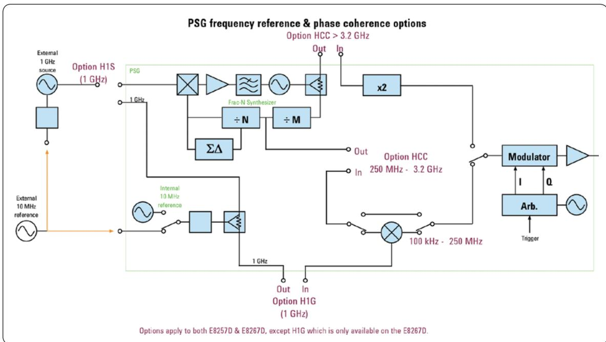
Figure 16. Option HCC provides access to PSGs LO from the rear panel for both low-band and high-band paths. Option H1S and H1G provide the ability to use a 1 GHz reference.
