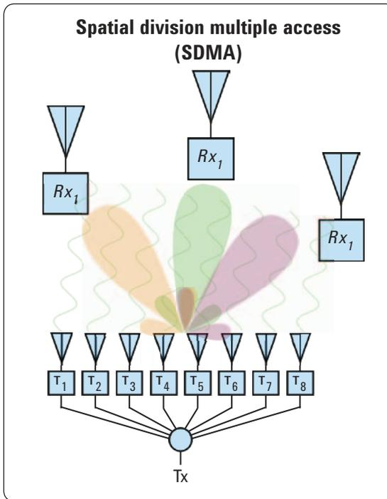
Figure 1d. An SDMA system uses beam forming to direct or receive energy only to or from a specific transmitter or receiver.
