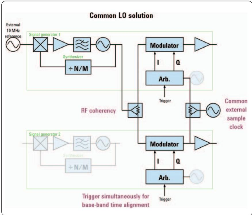
Figure 9. Sharing a common LO between signal generators effectively eliminates the relative phase errors between signals and provides full phase coherency. The LO may be provided by using an external source or by distributing the "master LO" of one instrument with other instruments.
