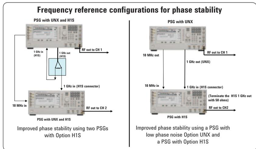
Figure 11. PSGs Options H1S, H1G and UNX provide the ability to improve phase stability between instruments by locking the 1 GHz reference.
