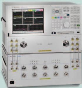
The Agilent U3022AE10 multiport test set, combined with two-port PNA, PNA-L or PNA-X network analyzer and Option 551, offers full crossbar and calibrated measurements up to 12-port.
