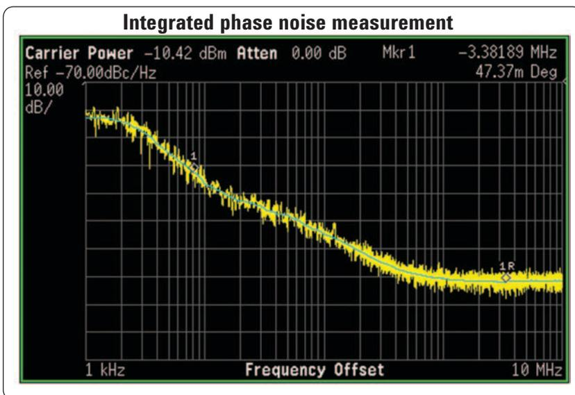
Figure 8. The total phase error due to phase noise between signal sources can be determined by integrating the uncorrelated phase noise with integration limits set equal to the bandwidth of the applicable signals used in the system.
