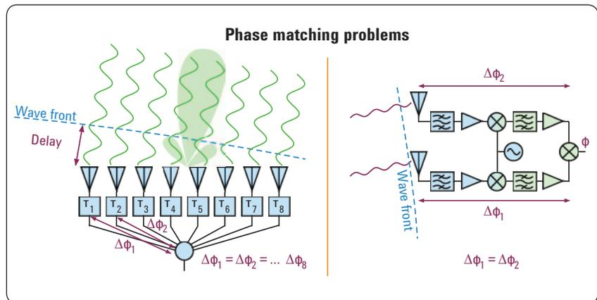
Figure 2. Coherent multi-channel systems often require phase matching between channels.
