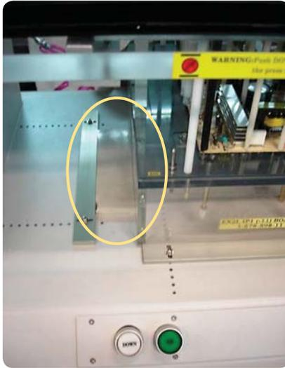
Figure 7. Spacer bar added between bar and fixture.
