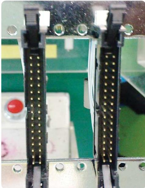
Figure 2. 34-pin male connector on flat cables
