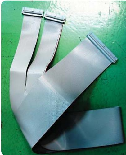
Figure 5. 64-pins to 32-pins split flat cable
