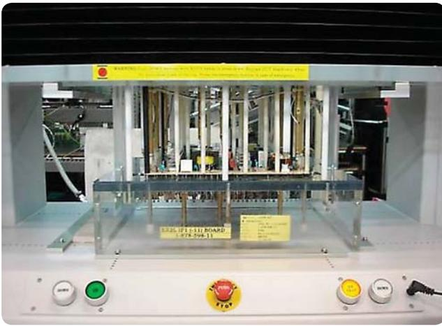
Figure 10. Fixture engaged with 2/3 probe compression.
