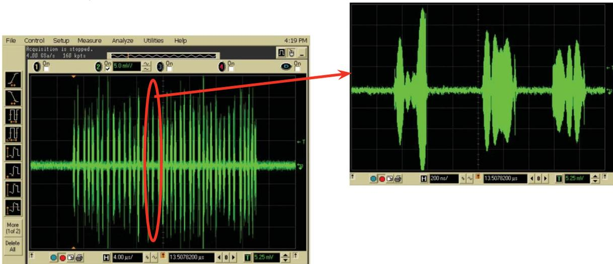
Figure 25. A view of the impulse noise
