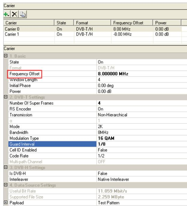
Figure 17. DVB-T/H interference generation
