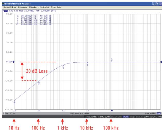
Figure 12. Transmission characteristic of pulse transformer (PN 5188-4425)
