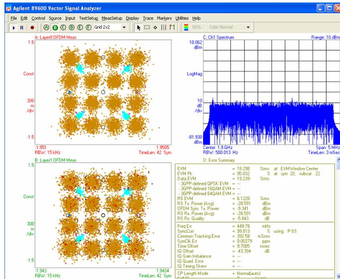
FIGURE 3: The four-channel MIMO measurement results from a downlink RF transmitter.
