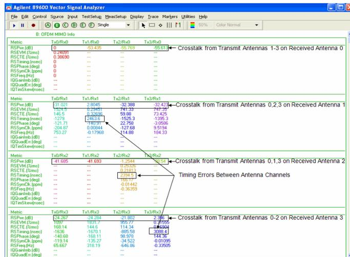
FIGURE 4: According to this VSA MIMO Information table, timing errors exist between the antenna channels. This is problematic since timing errors which approach or exceed the LTE cyclic prefix duration (4.69  $\mu$ s) can ultimately impact measurement accuracy.
