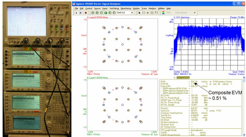
FIGURE 2: The four-channel MIMO test setup shown on the left consists of four Agilent signal generators and arbitrary waveform generators and a four-channel 90000X oscilloscope, while a baseline measurement result using the oscilloscope is shown on the right.
