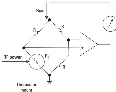
Figure 3. Bridge technique used in thermistor sensor
