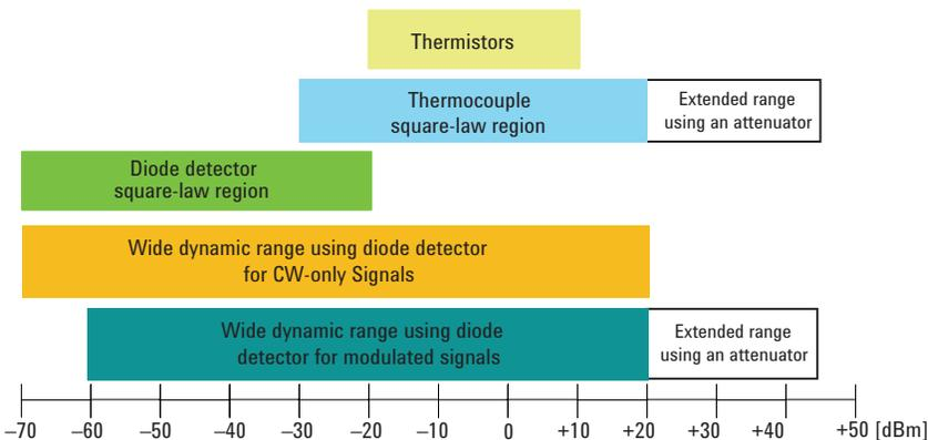
Figure 10. Power range of various sensor types
