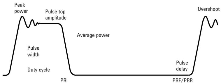
Figure 2. Typical radar pulse characteristics
