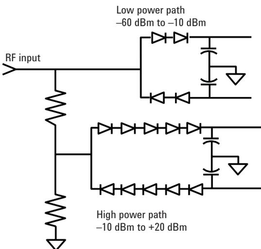
Figure 7. Schematic of a diode-attenuator-diode sensing element
