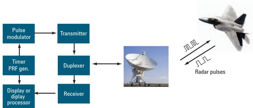
Figure 1. Block diagram of a simple radar system
