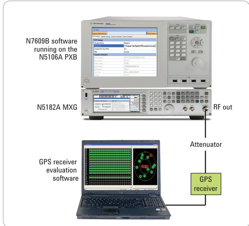
FIGURE 1: Shown here is a typical GPS receiver test setup with the N7609B. The baseband GPS signal is created by the N7609B running on the N5106A PXB, upconverted to RF by the MXG and sent to the GPS receiver. The GPS receiver output is then sent to evaluation software on a PC.
