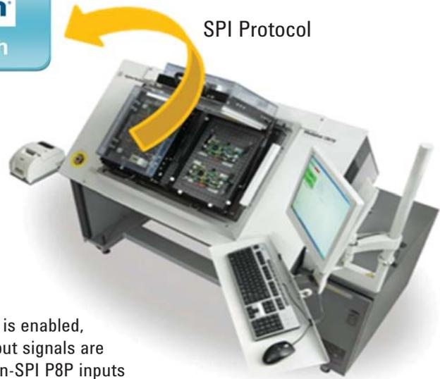
**Figure 1. PCM SPI Flash programming on Agilent Medalist i3070 in-circuit tester**
