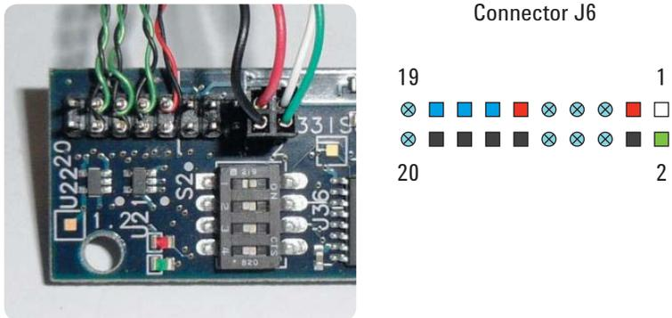
Figure 1. Connections on CET card (J6 connector)
