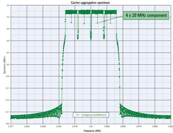
Figure 19. Carrier aggregation spectrum of four component carriers
