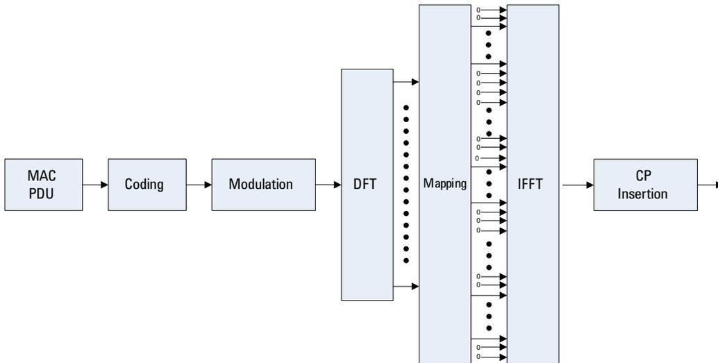
Figure 4. Enhanced uplink multiple access block diagram
