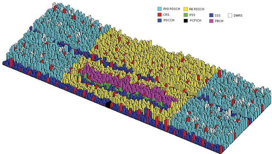
Figure 10. Example of resource block allocation in LTE-Advanced
