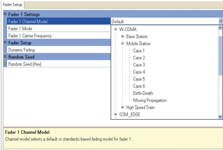
FIGURE 5: Shown here are predefined mobile station fading models for W-CDMA.
