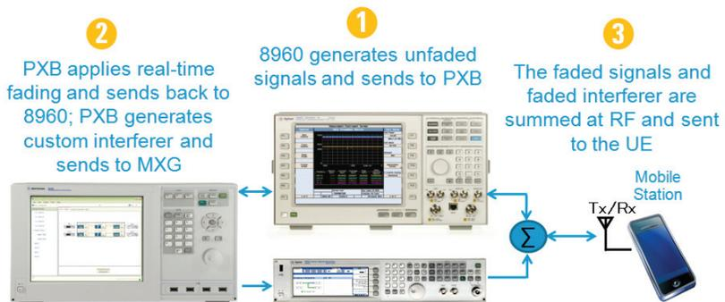
FIGURE 3: With the single channel with custom interferer test configuration, the PXB applies real-time fading to the 8960 and generates custom interferers.
