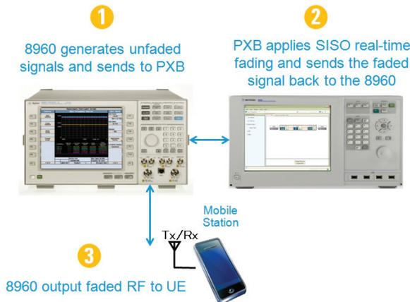
FIGURE 2: With the single-channel (SISO) test configuration, single-channel fading is applied to the 8960 for user equipment testing.
