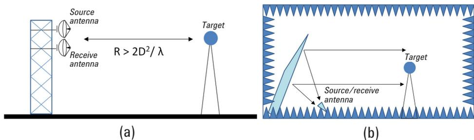
Figure 7. There are two common forms of RCS test facilities: outdoor far-field (a) and compact anechoic chambers (b)
