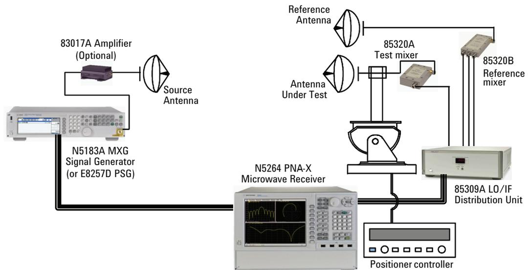
Figure 2. Far-field remote-mixing configuration using Agilent's MXG signal generator and N5264A microwave receiver
