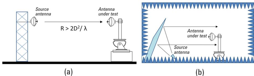
Figure 1. The most common forms of far-field test facilities are outdoor (a) and compact indoor (anechoic chamber) (b)
