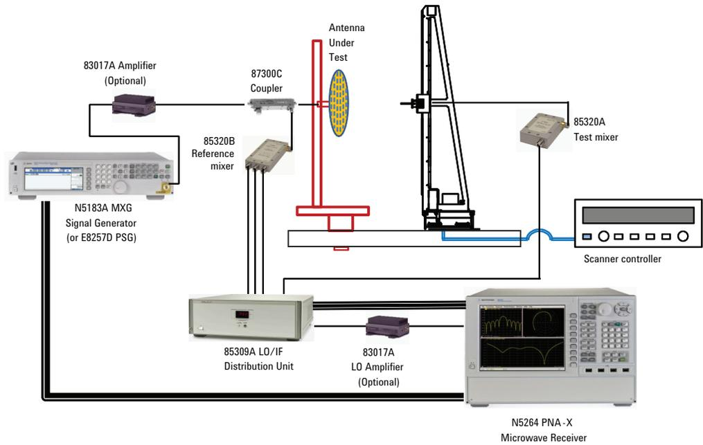
Figure 6. Near-field configuration for remote mixing technique using the Agilent MXG and N5264A microwave receiver
