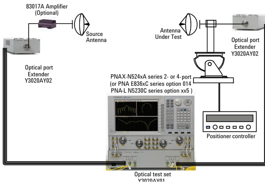
Figure 3. Far-field configuration using the Agilent PNA-X and optional optical extenders for larger facilities
