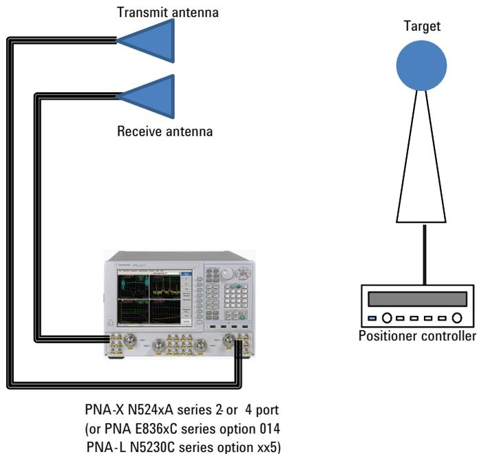
Figure 8. RCS configuration using the Agilent PNA-X
