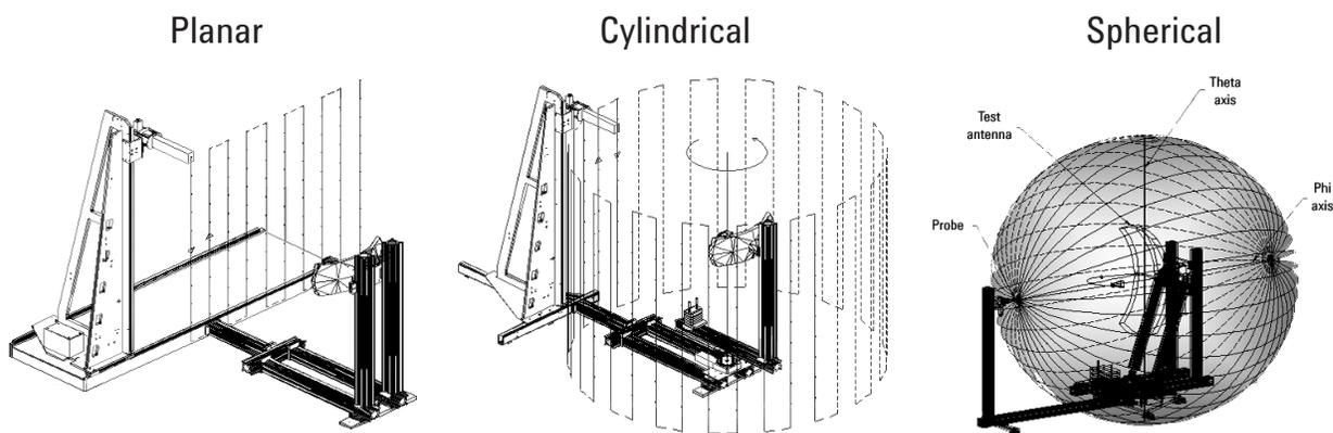
Figure 4. The three common forms of near-field test facilities are planar, cylindrical and spherical
