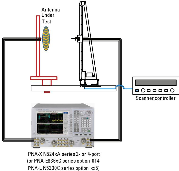
Figure 5. Basic near-field configuration using the Agilent PNA-X
