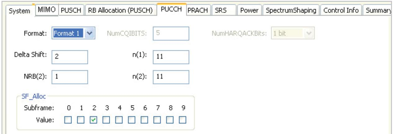
Figure 31. GUI of PUCCH parameters of LTE-Advanced UL MIMO source
