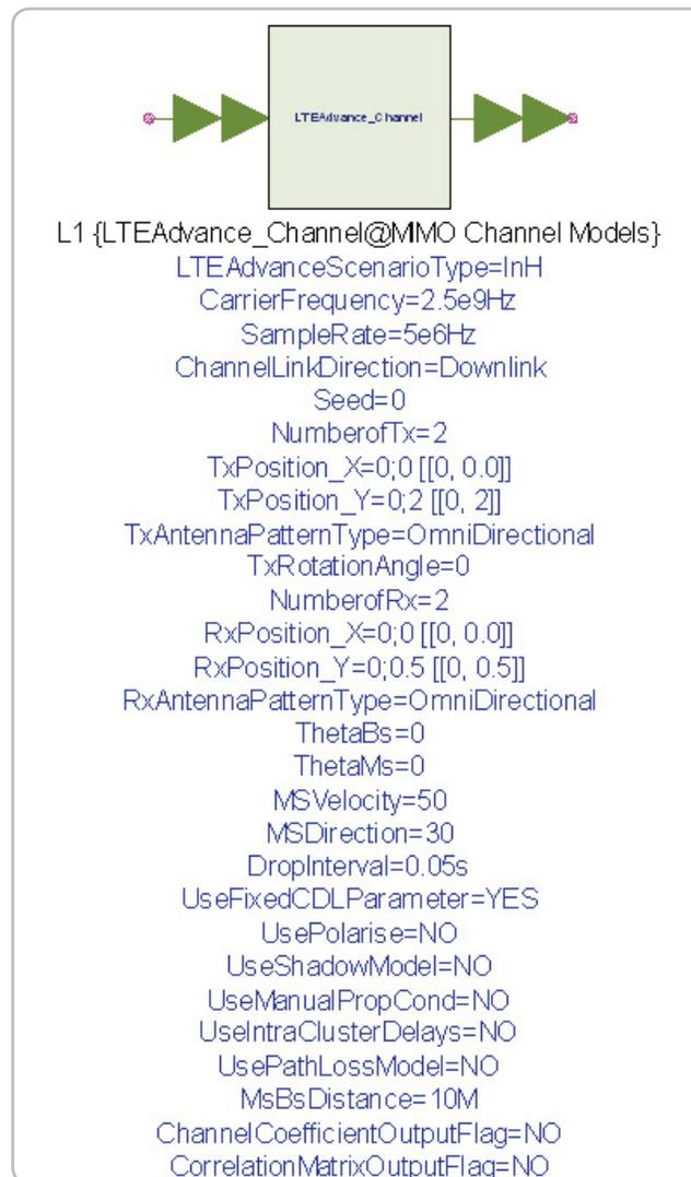
Figure 37. LTE-Advanced MIMO channel model in SystemVue
