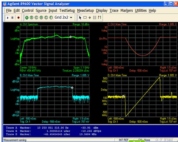
Figure 6. Spectrum, time waveform, phase and group delay measurements of an LFM UWB radar signal
