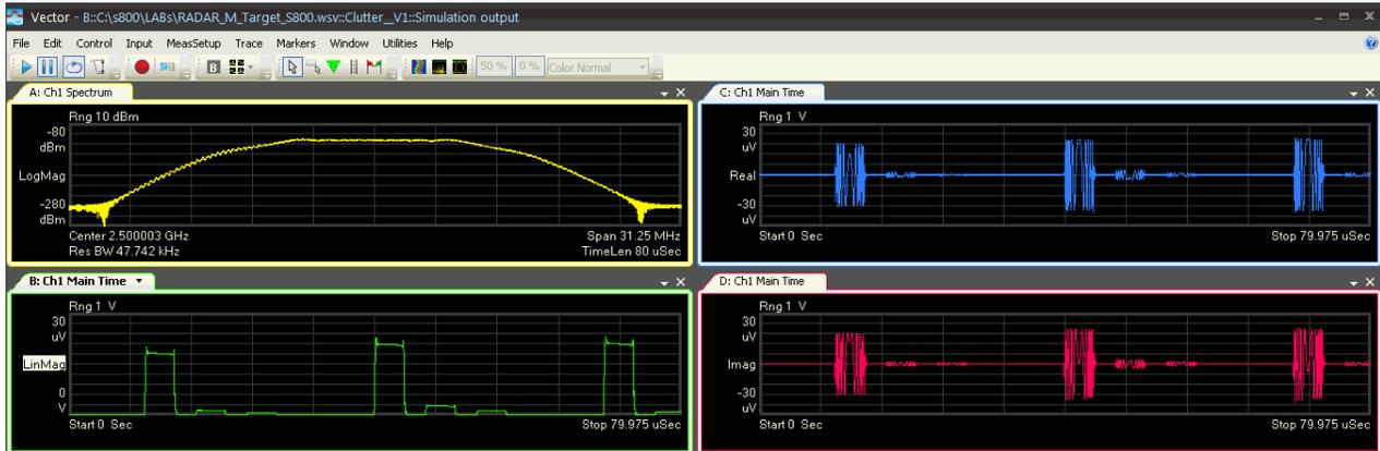
Figure 4. Generated radar test signals: received spectrum (yellow); and radar target returns with clutter, displayed as amplitude (green), real part (blue) and imaginary part (red)
