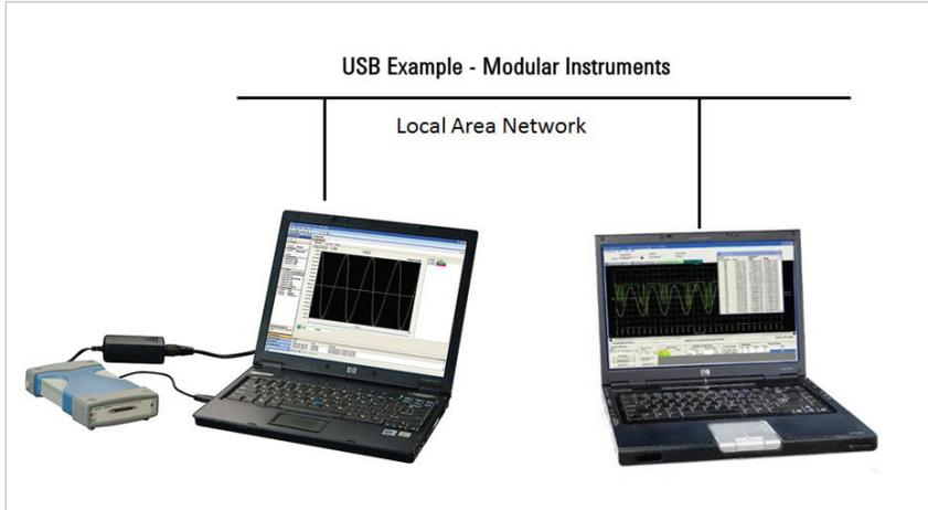
*Figure 6. The Agilent U2700A USB-Enabled modular instrument accessed via remote pc-to-pc connection*
