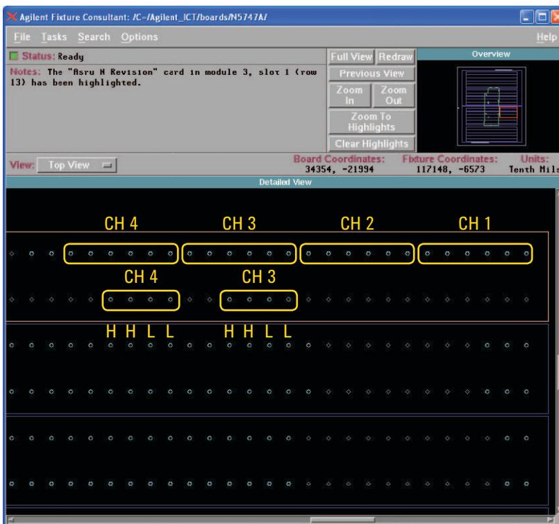
Figure 6. Fixture consultant view of DUT power supply channels on ASRU-N card.
