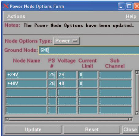
Figure 11. Defining N5747A power supply (connected to utility card) in board consultant.
