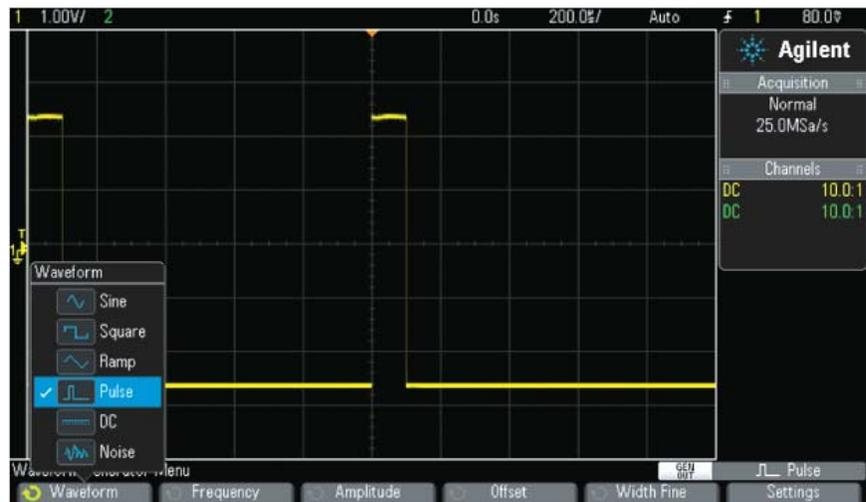
Figure 1: The integrated function generator in the Agilent 2000 and 3000 X-Series oscilloscopes uses the oscilloscope's large display to set up the waveform and saves space and money compared to a stand-alone function generator.
