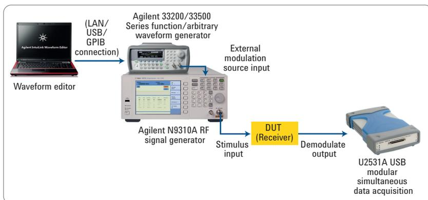
Figure 1. A typical system setup for measuring ASK/FSK receivers
