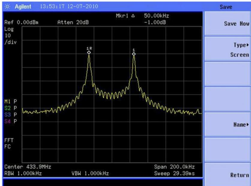
Figure 10. View an FSK signal in spectrum analyzer mode
