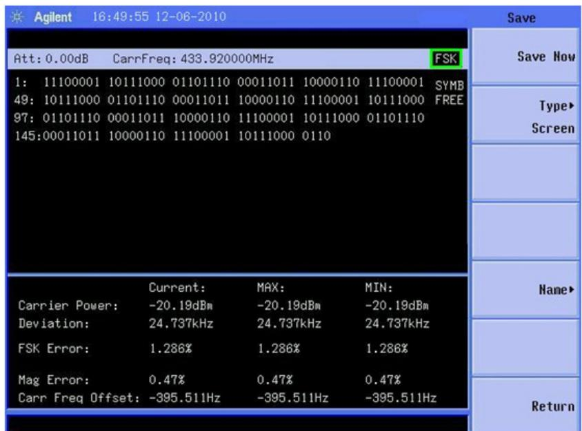
Figure 12. FSK demodulation – symbol view
