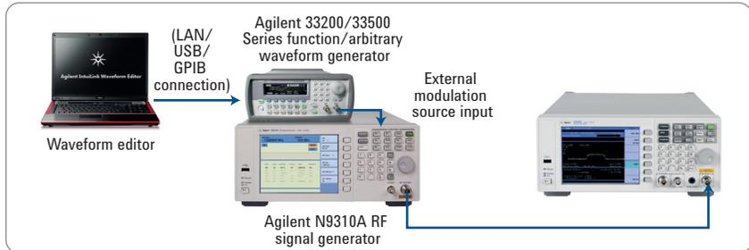
Figure 3. Equipment configuration for FSK signal generation and measurement
