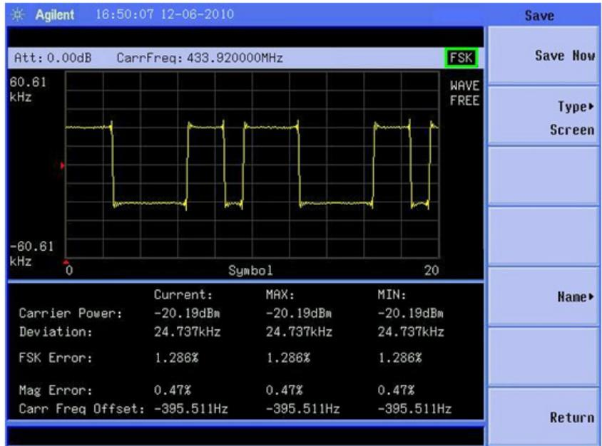
Figure 11. FSK demodulation – waveform view
