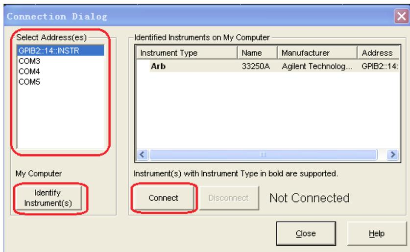
Figure 8. Choose the instrument address and press "Connect"
