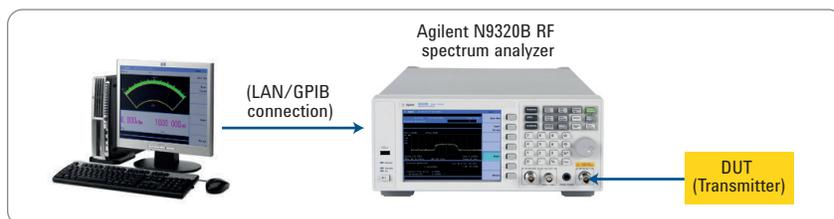
Figure 2. A typical system setup for measuring ASK/FSK transmitters
