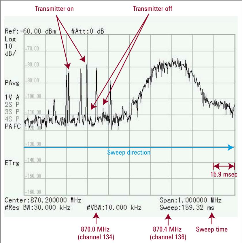
Figure 2. Over-the-air measurement of a GSM 850 downlink transmission using the Agilent N934xC HSA with attached antenna
