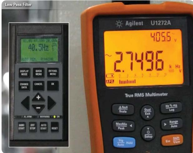
Figure 4. Inaccurate VFD output frequency measurement without low pass filter
