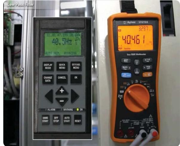
Figure 5. Accurate VFD output frequency measurement with low pass filter
