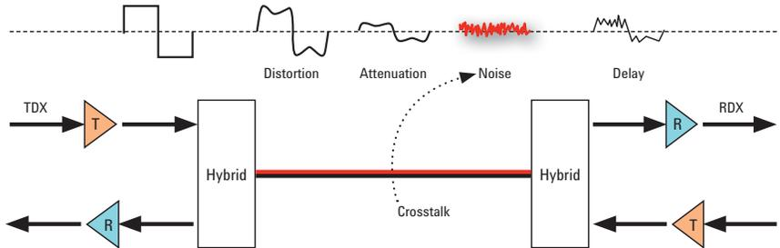
Figure 7. Noise, with different crest factors, can be added to emulate real conditions
