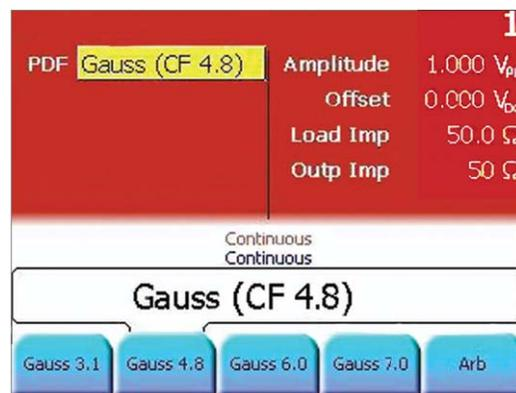
Figure 8. Push button selection of the noise crest factor
