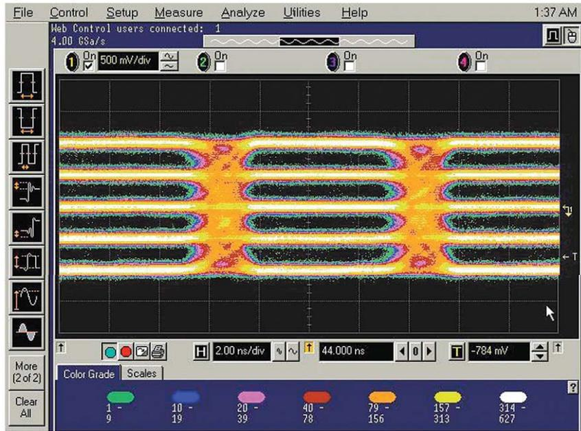
Figure 9. PAM5 signal with 0.1Vpp noise
