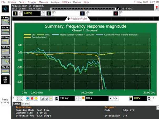
Figure 2-2. This custom probe system has a response that is far from flat.
