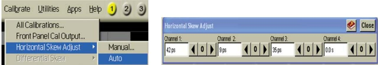
Figure 3. Dialogue boxes for horizontal de-skew of channels. Dialogue to select Auto or Manual is on the left. Manual adjustment dialogue is on the right.
