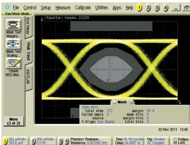
Figure 17. Typical eye diagram with mask margin.
