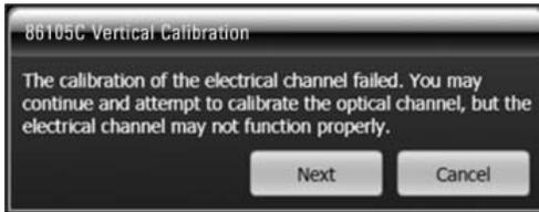
Figure 21. Dialogue box for reference receiver calibration and failure of electrical calibration.
