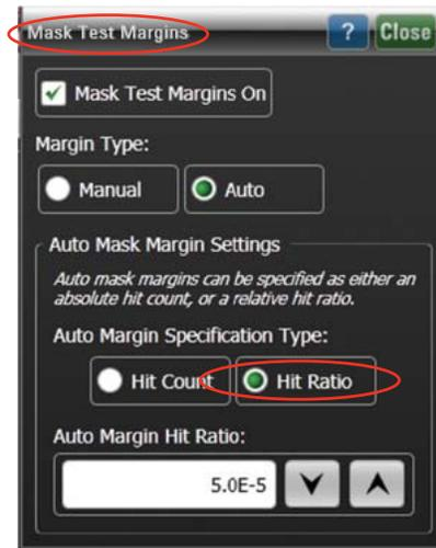
Figure 16. Mask Test Margins dialog box to enable mask margins and Hit Ratio.
