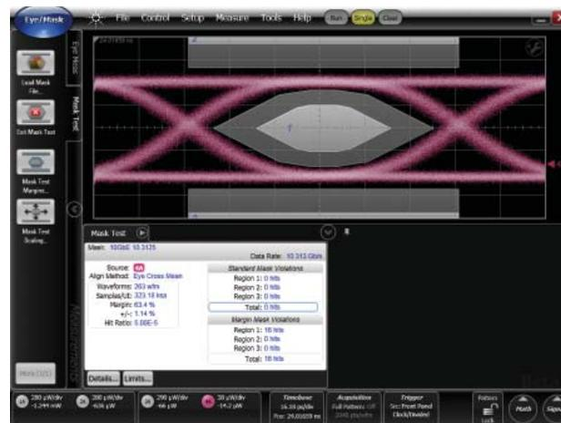
Figure 17. Typical eye diagram with mask margin.
