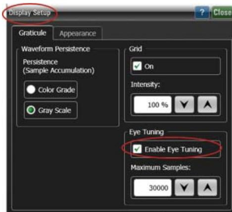
Figure 6. Display dialogue box to enable Eye Tuning mode.
