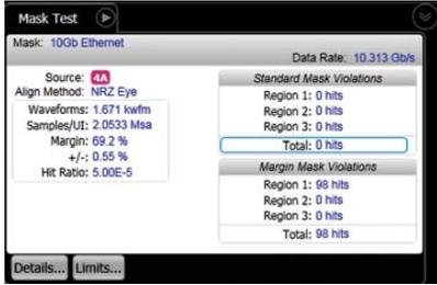
If the production batch of transceivers proves to have a mask margin much greater than what is needed by the customer, then fewer samples can be acquired. If the production batch is very close to specification and care must be used to assure that transceivers pass incoming inspection at the customer facility, then more samples are acquired.
