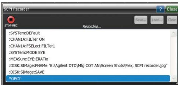
Figure 19. Dialogue box for the SCPI Recorder (firmware A.01.60 or later).
