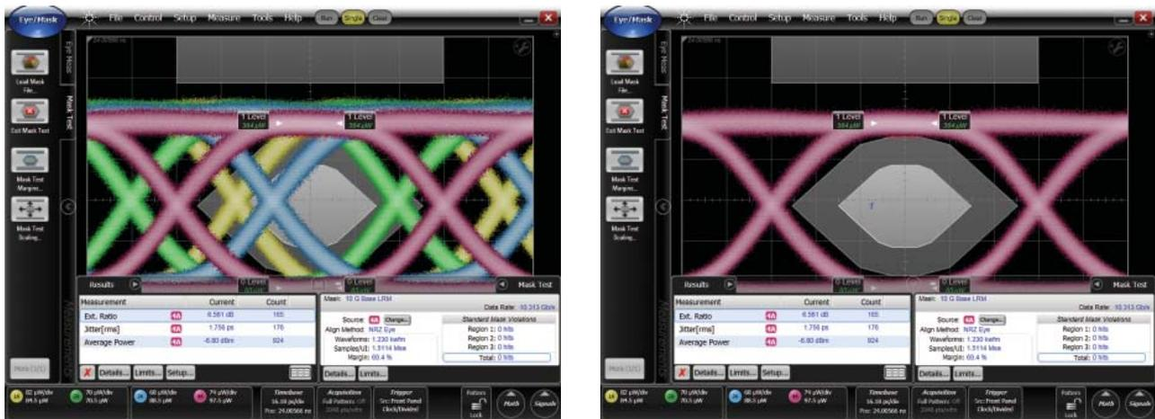
Figure 20a and b. Typical measurement results showing all channels and only one of the parallel channels.
