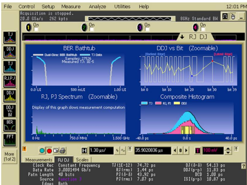
Figure 4. TJ measurement and its components – RJ, PJ, DDJ
