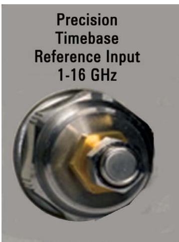
Figure 13. The 86108 Precision timebase reference input
