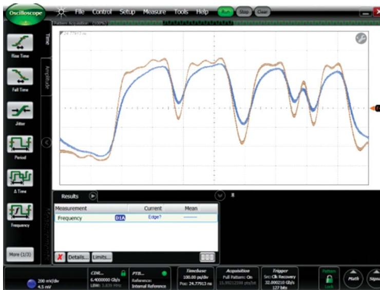
Figure 11. 86100D-SIM InfiniiSim-DCA provides a very fast and easy means to de-embed the effects of the module transmission lines
