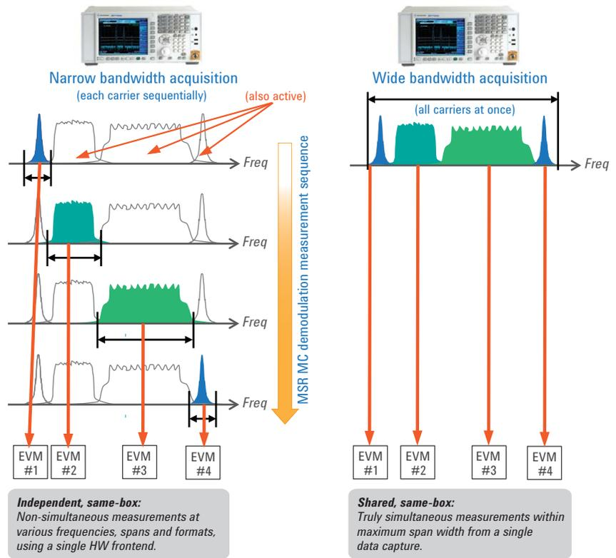
FIGURE 4. This image compares the use of sequential acquisition of each carrier using narrow bandwidth hardware on the left with the use of simultaneous acquisition of all carriers using wide bandwidth hardware on the right, for modulation analysis.
