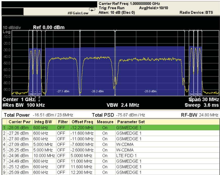
FIGURE 3. Shown here is a swept-spectrum view of a carrier-channel power measurement for one of the MSR conformance testing defined in 3GPP TS37.141.
