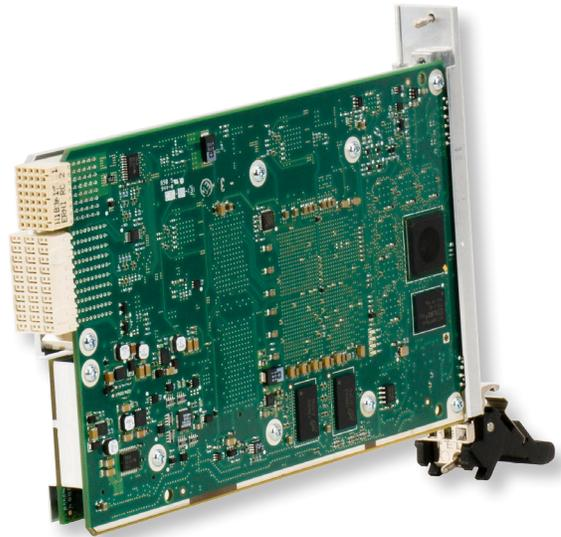
Figure 4b. PXIe connector style.
