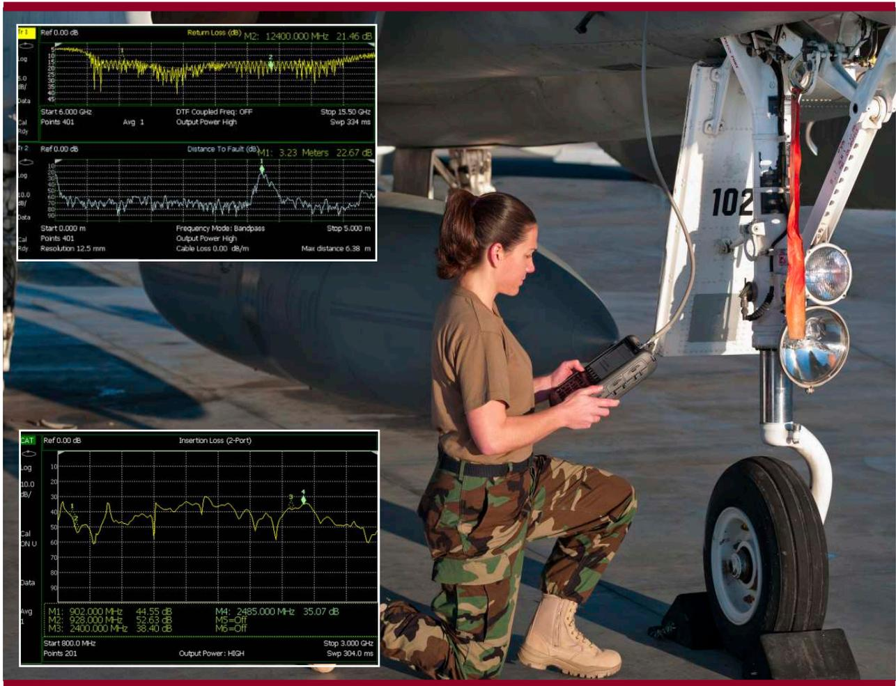
This application note introduces the practical aspects of cable and antenna testing, interpreting measurement results and instrument operation including calibration options such as CalReady and QuickCal using FieldFox configured as a cable and antenna analyzer. Measurement examples are provided showing techniques for measuring insertion loss, return loss, and locating faults in a transmission system.
