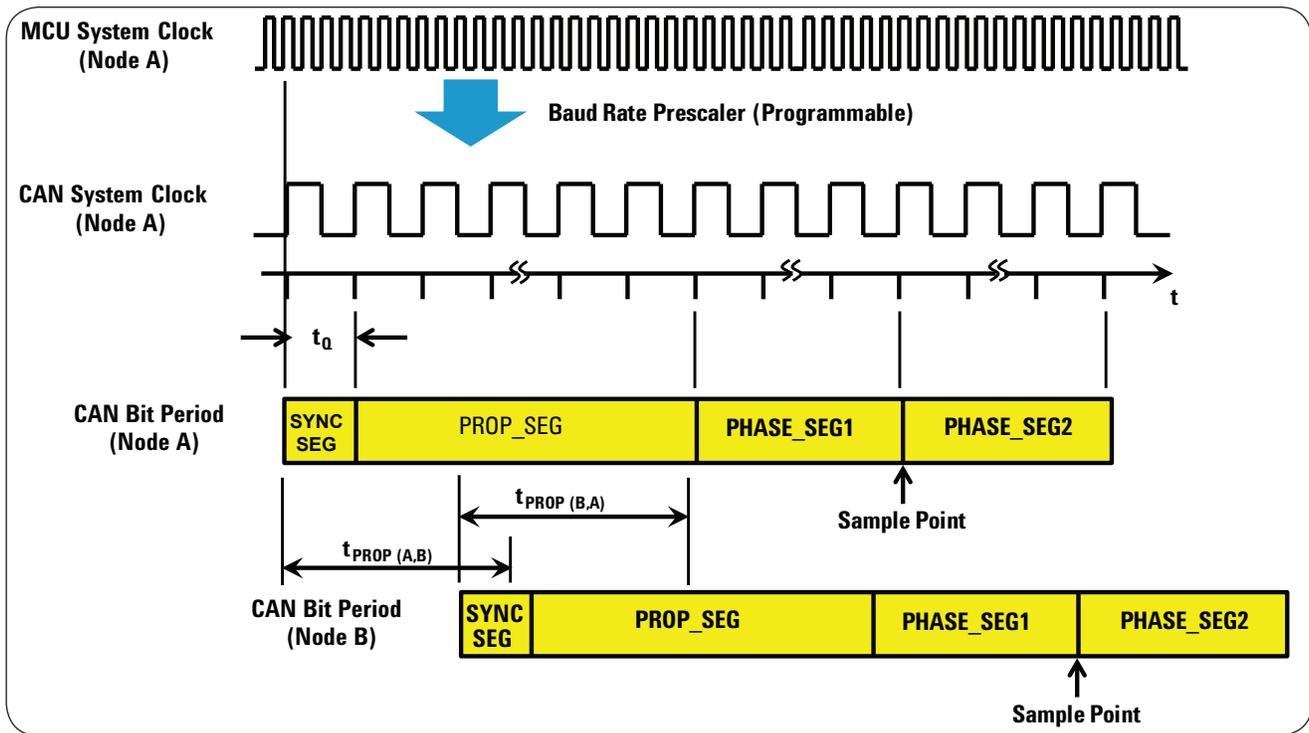
Figure 5: CAN bit-timing diagram for two widely-spaced nodes.
