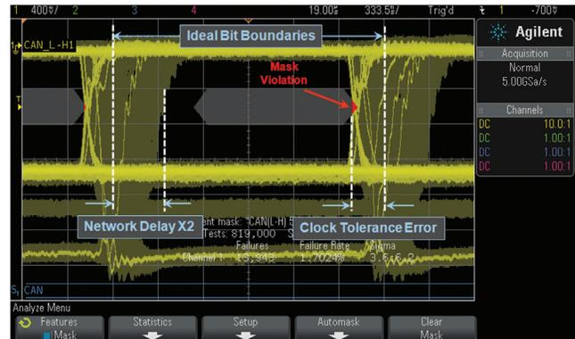
**Figure 7: Eye-diagram display showing system propagation delays AND edge shifts due to accumulated clock tolerance errors.**
