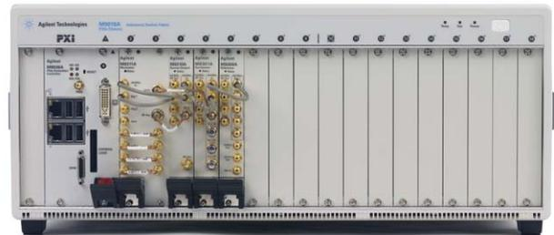
Figure 1. Agilent M9381A PXIe VSG (includes M9311A, M9310A and M9301A) pictured with M9300A frequency reference, M9036A embedded controller in a M9018A 18-slot chassis.
