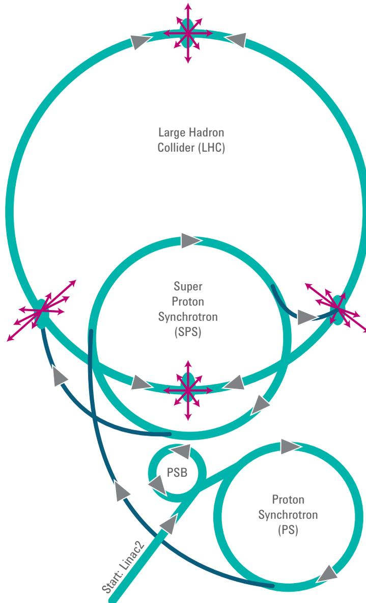
FIGURE 1. Simplified diagram of the LHC multi-stage synchrotron that accelerates protons to nearly light speed
