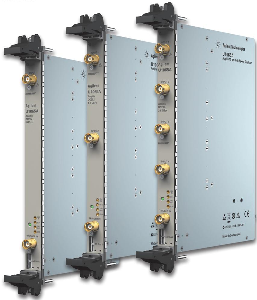
FIGURE 2. U1065A Acqiris 10-bit high-speed cPCI digitizers can be configured with one, two or four input channels and sampling rates of 2 to 8 GSa/s.
