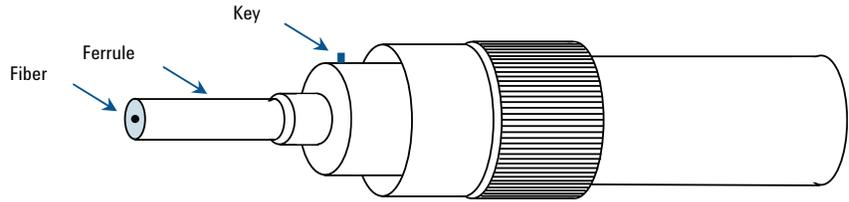
Figure 2. Optical Connector
