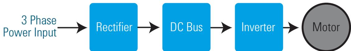
Figure 1. VFD block diagram
