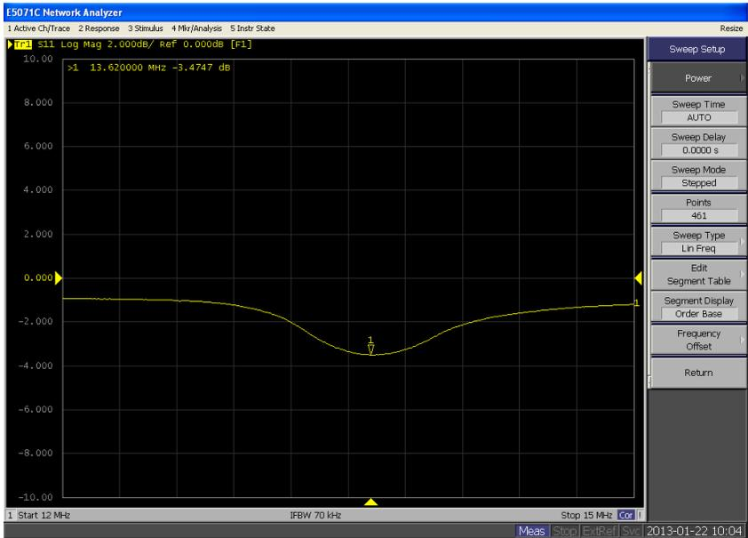
Figure 6. Return loss result measured with E5071C ENA
