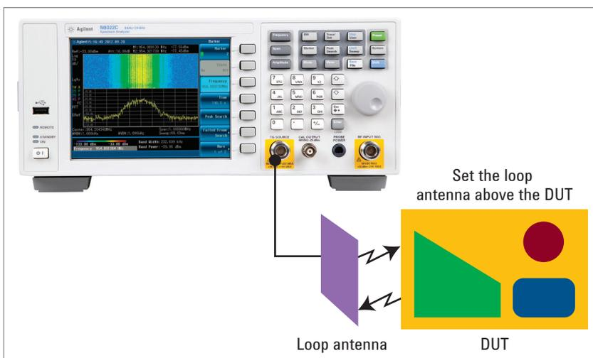
Figure 2. Simple test setup for reflection measurements
