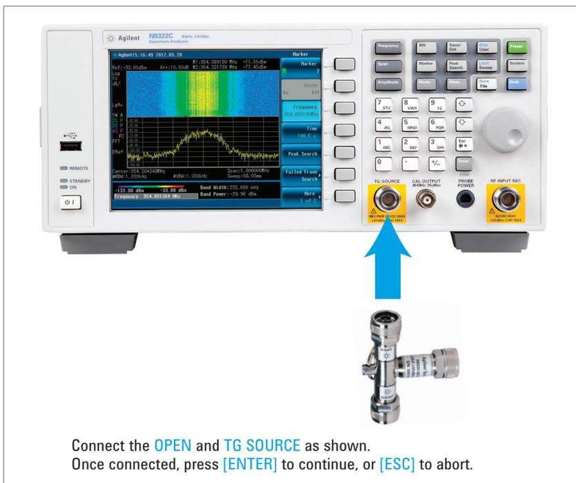
Figure 3. Performing OSL calibration on the N9322C BSA
