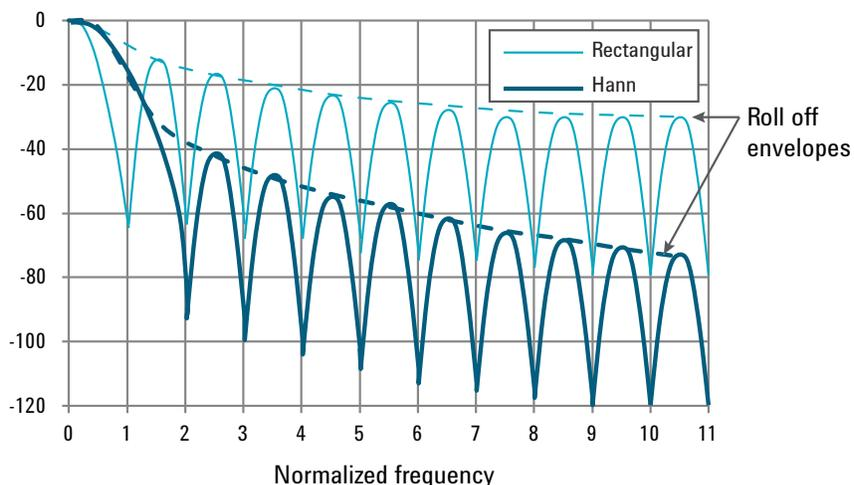
Figure 4-1. Rectangular and Hann window filter response characteristics
