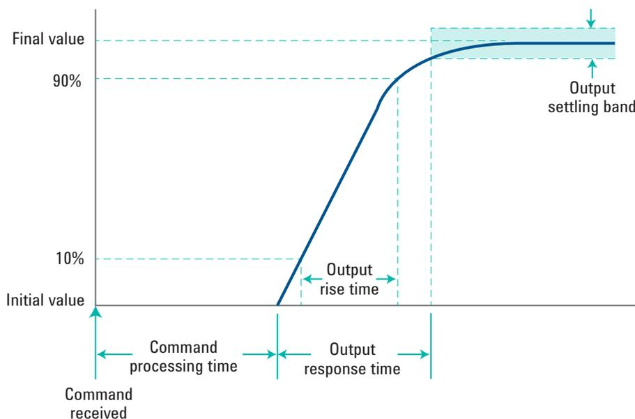
Figure 2-1. Power supply up-programming response time
