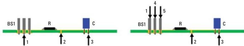
Test generated only for R and C. No test is generated for BS1(Terminals) because all its pins are on the same NET
