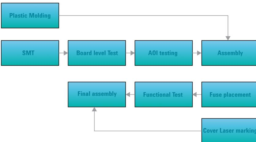
The process begins with surface mounting of the components and fuse terminals onto the printed circuit board. The printed circuit board is usually built in a panel of multiple boards to cater for lower manufacturing cost.
