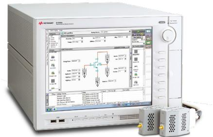
The B1500A supports the QSCV measurement by the Source/Monitor Unit (SMU). It enables the advanced step voltage QSCV method by the superior low current measurement down to 0.1 fA resolution and the intrinsic precise timing control. In addition, the B1500A and the application test for QSCV measurement implement the leak and offset compensations applicable to leaky device measurement as described later.
