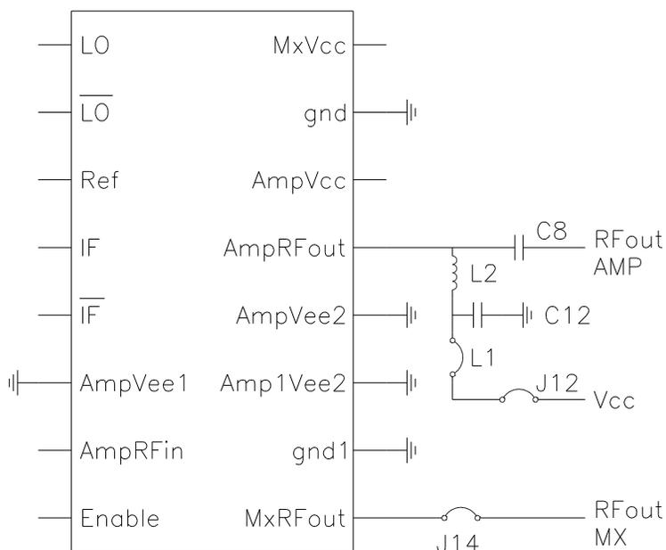
Figure 8. Detail of the demonstration board circuit with output network for 1500-2500 MHz operation. Component values are listed in table 4. Note: C12 is moved along the printed inductor (L2) to tune the output for minimum VSWR. See figure 3 for approximate C12 positions. L1 (shown in figure 3) is replaced with a jumper.
