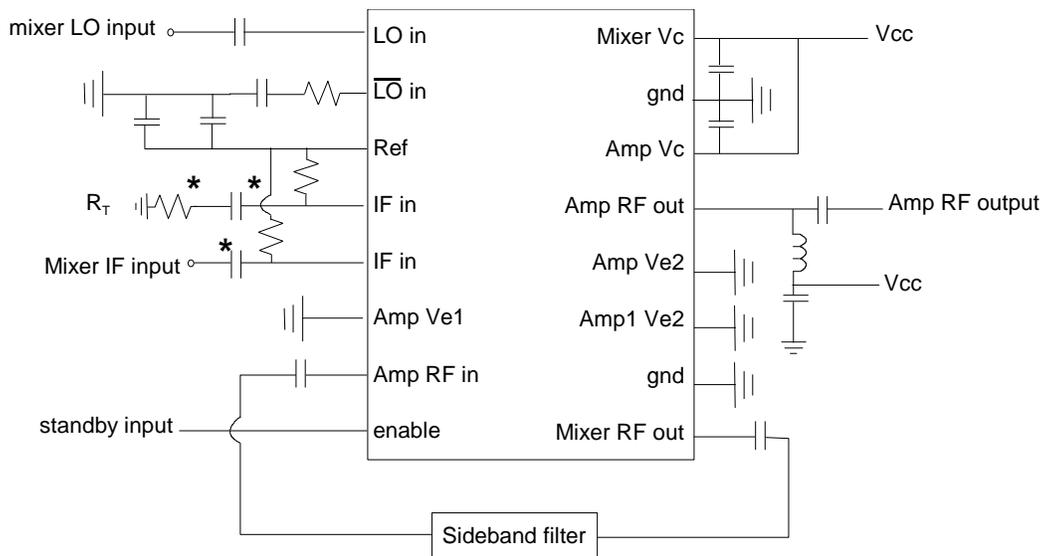
Figure 1. Typical application circuit for the HPMX-2006 upconverter/amplifier IC. Component values match those of test board- refer to table 4.  $R_T$  (optional) should be the same value as the IF source impedance. Asterisks indicate off-board components.
