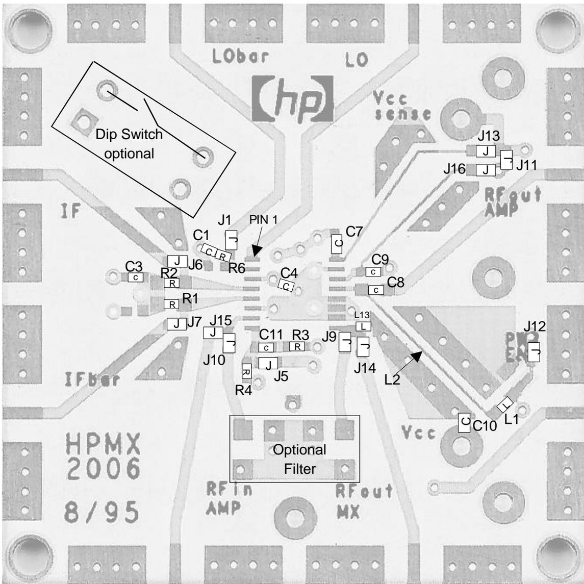
Figure 5. Component placement on the demonstration circuit board. The IC and SMA type connectors are not shown. Position of C12 along L2 will depend upon the intended output frequency. Figure 3 shows approximate positions for different frequencies. Note: C4 is mounted on the bottom side of the board- the solder mask will have to be removed from the pads in order to install C4. Component values are listed in table 4, board schematic in figure 4.
