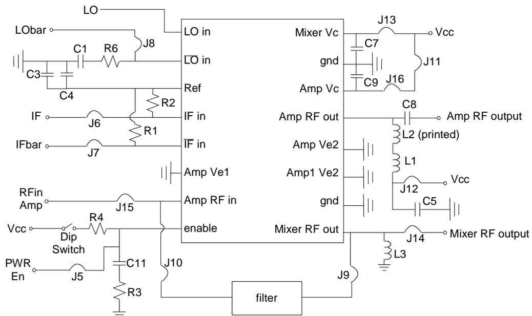
Figure 4. HPMX-2006 demonstration board schematic diagram . Amplifier output tuned at 900 MHz. Component values are listed in Table 4. Labels match those silk-screened onto the circuit board. See figure 5 for component placement on the board.
