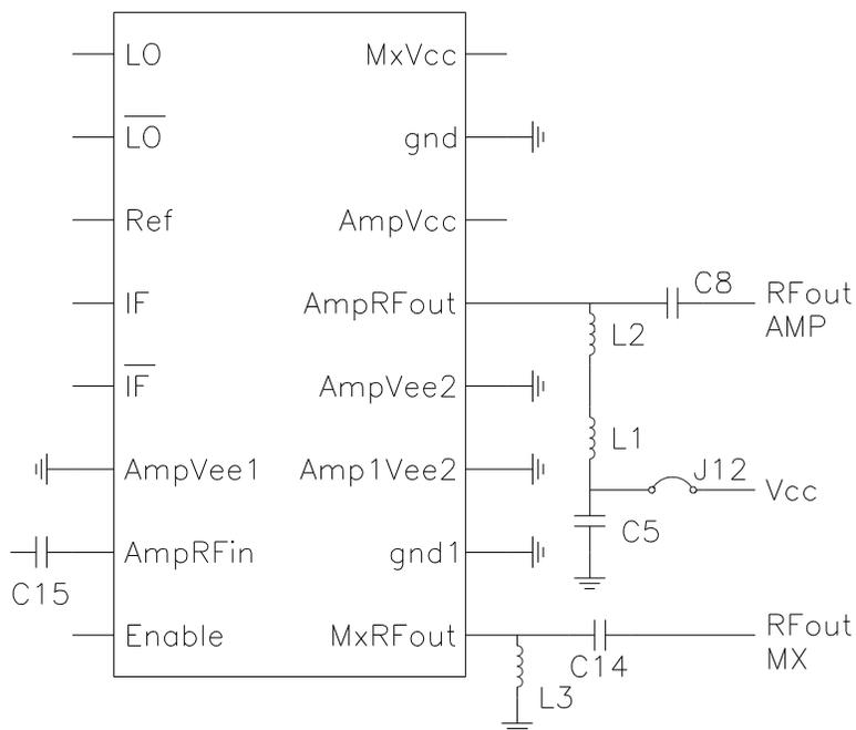
Figure 9. Detail of the demonstration board circuit with output network for 900 MHz operation. Component values are listed in table 4. C12 is not used. Note: C15 replaces J15 to tune the amplifier input. C14 replaces J14. L3 and C14 improve the mixer output VSWR.
