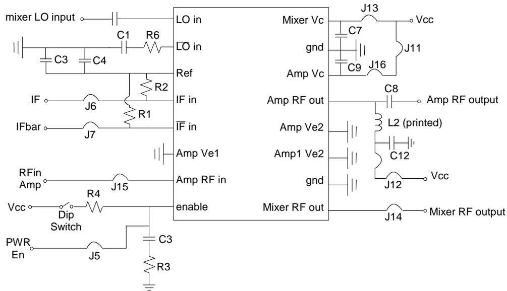
Figure 2. Schematic diagram of typical demo board use. Amplifier output tuned at 1500-2500 MHz. This schematic corresponds to the component placement diagram figure 3. Component values are shown in table 4. Note: L1 (shown in figure 4) is replaced by a jumper. C12 is used to tune the output at any specific frequency, by moving it along printed inductor L2. R3, R4 and C11 are optional components to allow dynamic testing of the chip enable function.
