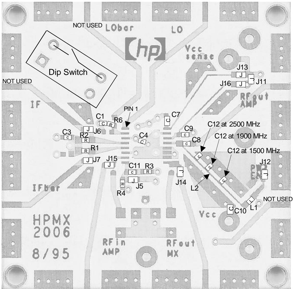
Figure 3. Typical demonstration test circuit board component placement for 1500-2500 MHz test board shown in figure 2. C12 positions along L2 are approximate - accurate placement should be determined by the board user. L1 is replaced by a 0Ω jumper. Note: C4 mounts on the bottom of the board. The solder mask will have to be removed from the pads to mount C4.
