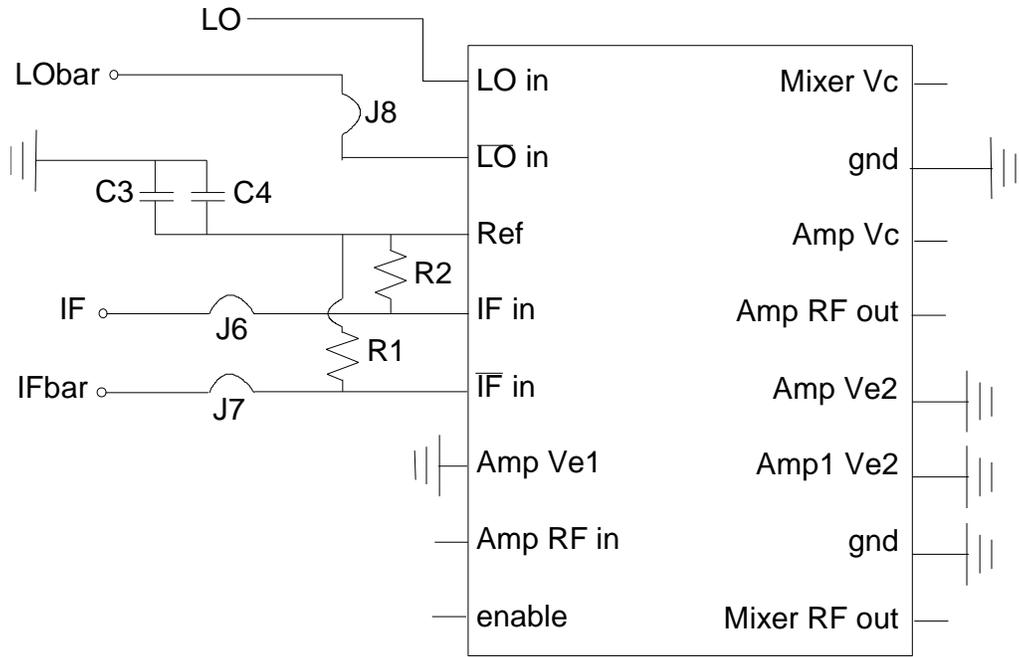
Figure 6. Detail of circuit options showing how to use balanced (differential) mixer LO and IF input lines. Component values are listed in Table 4.
