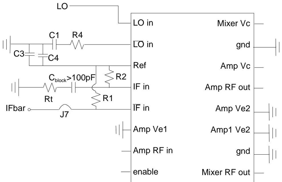
Figure 7. Detail of circuit options showing how to use unbalanced (single-ended) mixer LO and IF input lines. Component values are listed in Table 4. Rt is optional, should be the same value as the IF source impedance.
