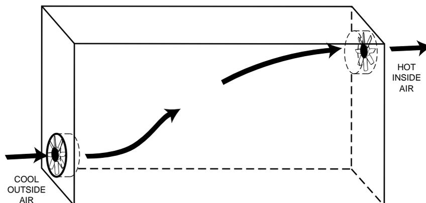
Figure 1. Use of Fans to Augment Convection Cooling.
